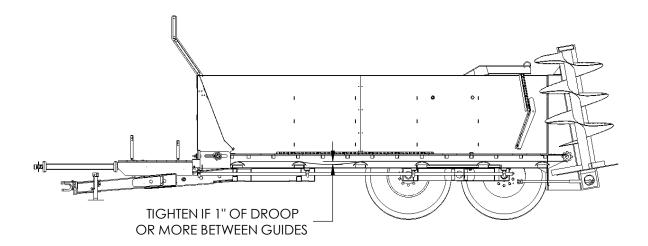
**BE SURE TO KEEP PROPER TENSION ON APRON CHAINS.** The (2) Apron Chain tightener bolts are located in the front of the unit at each side of Apron Shaft. They should be adjusted evenly to help keep proper chain alignment.
