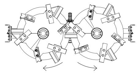
Beater teeth, knives, and/or scoops should be replaced in a manner that will keep the corresponding beaters as balanced as possible.
