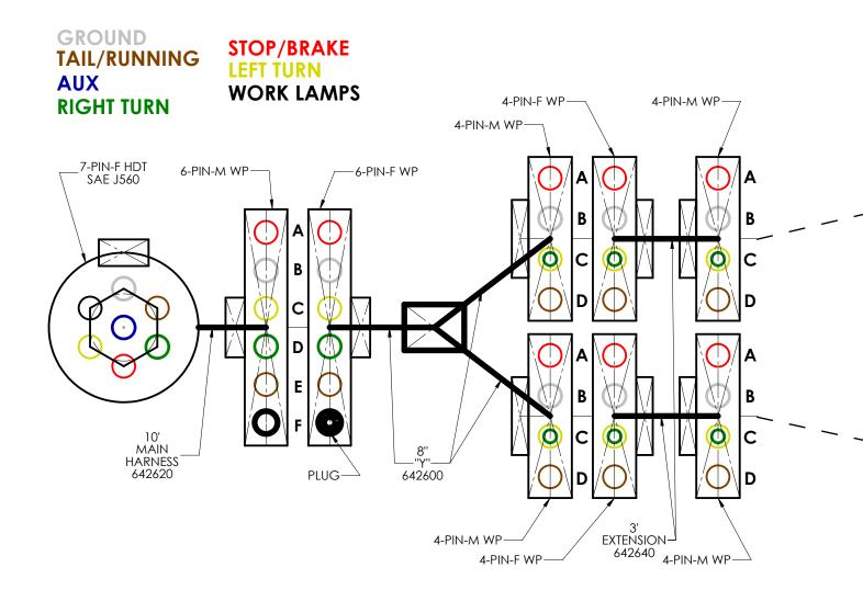
ALL END CONNECTORS ARE SHOWN LOOKING AT THE PIN SIDE WITH LOCKING TABS POINTING THE DIRECTION SHOWN
