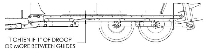
The (4) apron chain tensioner bolts are located in the front of the unit at each side of the (2) apron tensioner shafts. They should be adjusted evenly to help keep proper chain alignment. Measure from the front of the box weldment to the left and right extents of the tensioner shaft to ensure tension is being applied evenly. The apron tensioner bolts are double nutted to lock the position in place.
