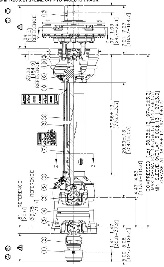
1000 RPM 1-3/8 X 21 SPLINE C-V PTO W/CLUTCH PACK
