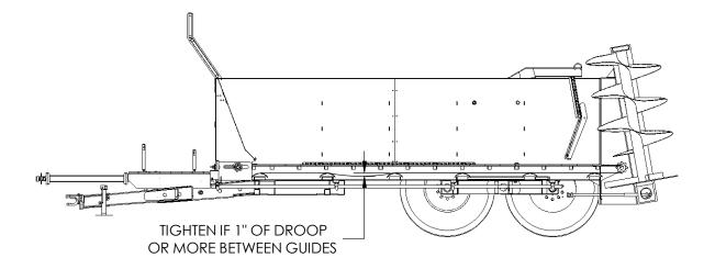
**BE SURE TO KEEP PROPER TENSION ON APRON CHAINS.** The (2) Apron Chain tightener bolts are located in the front of the unit at each side of Apron Shaft. They should be adjusted evenly to help keep proper chain alignment.
