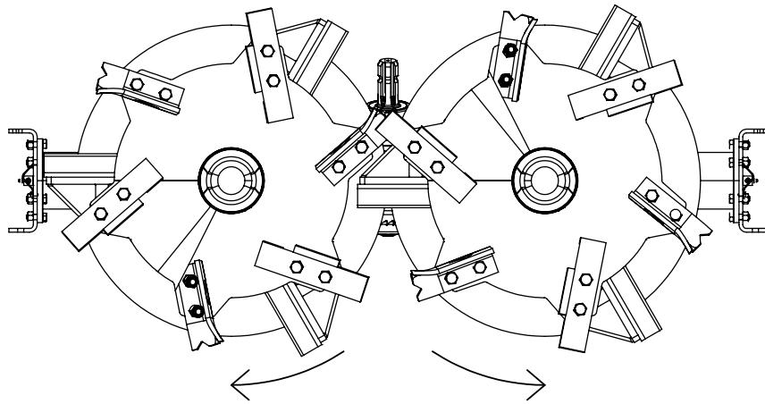
Beater teeth, knives, and/or scoops should be replaced in a manner that will keep the corresponding beaters as balanced as possible.
