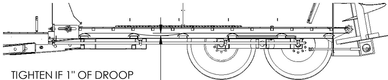
The (4) apron chain tensioner bolts are located in the front of the unit at each side of the (2) apron tensioner shafts. They should be adjusted evenly to help keep proper chain alignment. Measure from the front of the box weldment to the left and right extents of the tensioner shaft to ensure tension is being applied evenly. The apron tensioner bolts are double nutted to lock the position in place.
