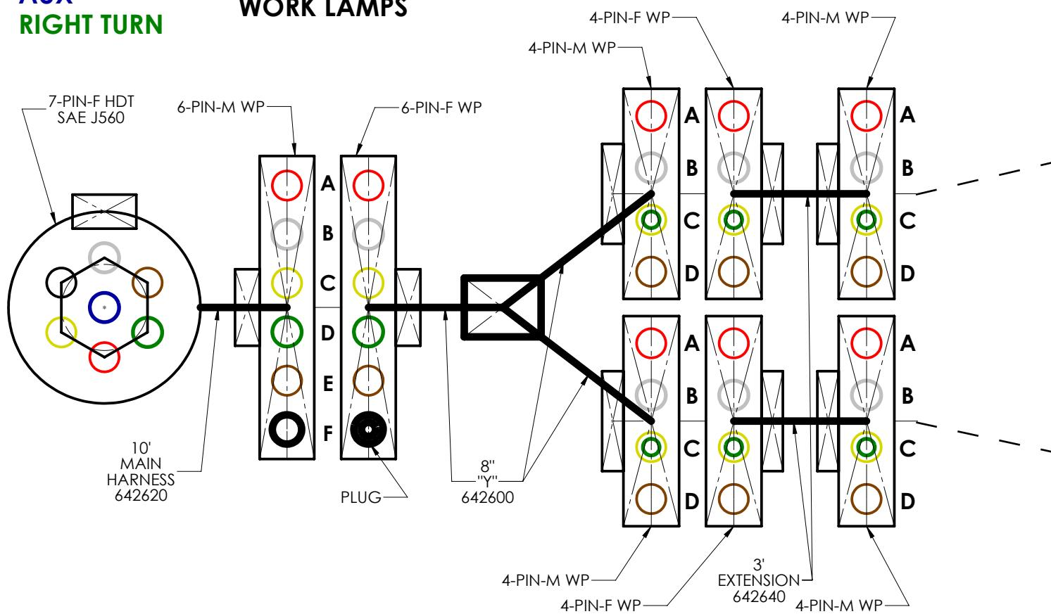
ALL END CONNECTORS ARE SHOWN LOOKING AT THE PIN SIDE WITH LOCKING TABS POINTING THE DIRECTION SHOWN
