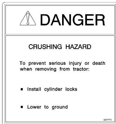
22 P/N: 487770 Danger, Crushing Hazard
