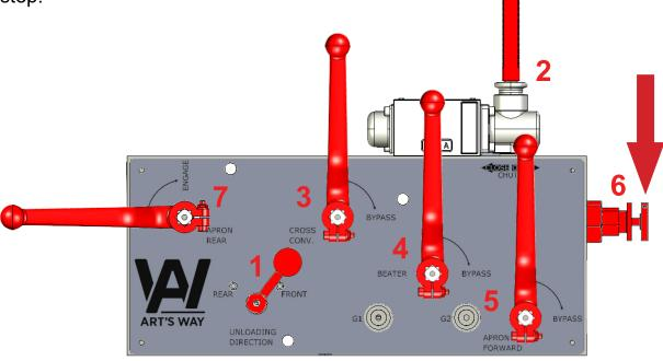
To stop the unloading process work your way backward with the lever order. First slowly turn the "APRON FORWARD" lever (5) 90 degrees to the "BYPASS" position. The apron chain will have stopped.
