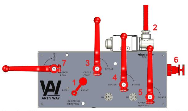
Finally, with everything moving material feed rate may be controlled by turning knob (6) slowly which will control the speed of the apron chain movement. Turn the outer knob counter clockwise to increase speed and clockwise to decrease speed. The inner knob can be used to lock the speed setting in place. Manifold levers should only be put into "BYPASS" or "ENGAGE" and should not be used to meter flow (speed). Once you have unloaded the forage box move to the next step.
