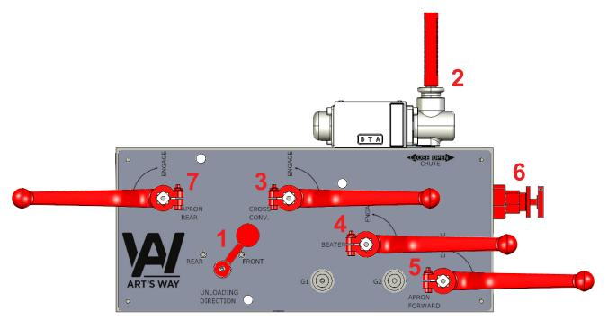
Ensure the cross conveyor lever is set to "BYPASS" and the cross conveyor chain has stopped before moving to the next steps. Failure to do so may result in damage to the unit. Once all functions have stopped you may now Shift the "CHUTE" handle (2) in the "CLOSE" direction shown. This will retract the cross conveyor chute cylinder and close the chute.
