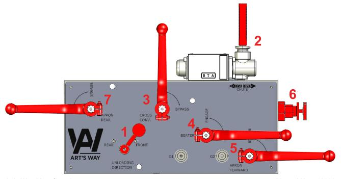
Next, with the cross conveyor moving, to start the beaters slowly turn the "BEATER" lever (4) 90 degrees to the "ENGAGE" position. The beaters will have started to move.
