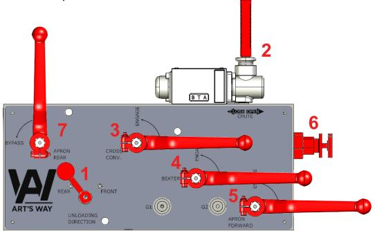
Slowly turn the "APRON REAR" lever (7) 90 degrees to the "BYPASS" position. The apron chain will have stopped moving. Now turn off hydraulic supply from tractor. The unit is now ready for the next load.
