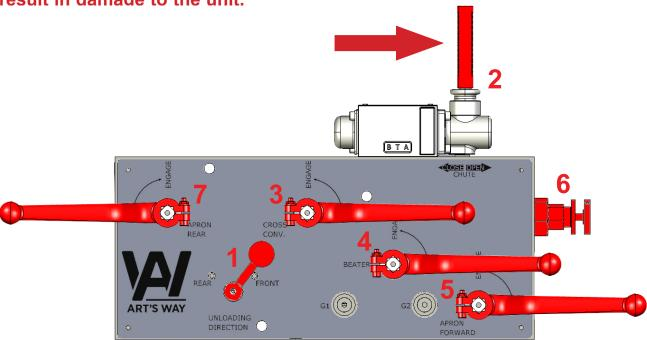
Next, to start the cross conveyor slowly turn the "CROSS CONV." lever (3) 90 degrees to the "ENGAGE" position. The cross conveyor will have started to move.
