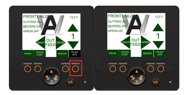
With the apron chain turned on you may now adjust the speed of the apron chain by pressing the buttons noted below.
