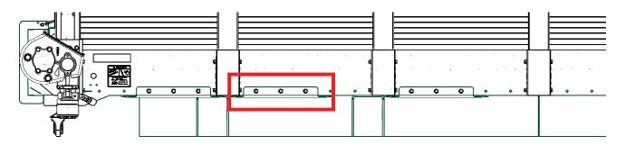
Tire bump stops are included with every Art's Way Forage box. You are responsible for re-positioning them in locations above tires for tandem / rocking style running gear. When installing ensure the gussets on the insides of the bump stops make contact with the "C" channel main frame members.
