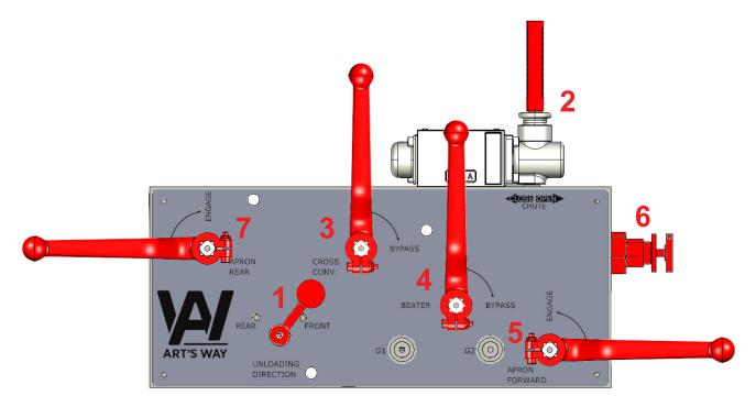
Next, with the cross conveyor and beaters moving, to start the apron chain slowly turn the "APRON FORWARD" lever (5) 90 degrees to the "ENGAGE" position. The apron chain will have started to move.
