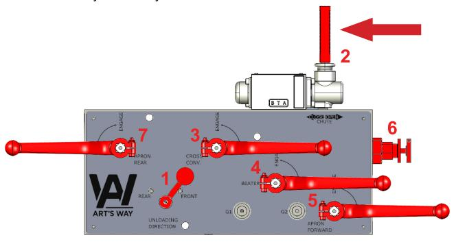
Now turn off hydraulic supply from tractor. The unit is now ready for the next load. It is highly recommended to stop/shut off hydraulic flow to the forage box in-between unloading cycles to prevent unnecessary heat buildup and wear.
