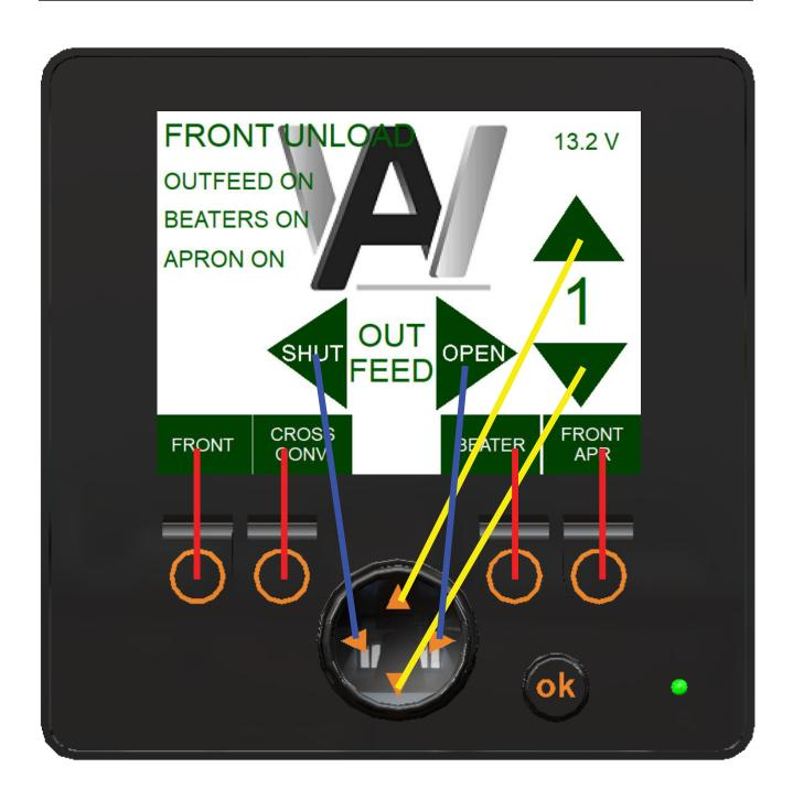
The above diagram illustrates what control labels correspond with each physical button. The "ok" button is used to access a settings menu. This menu can be assessed by pressing and holding the "ok" button for 5 seconds. Only access the settings menu when all operations are stopped and hydraulic power is turned off.
