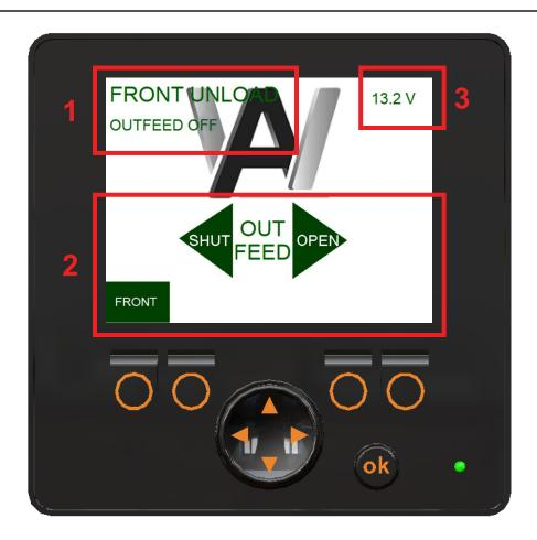
The canbus operational display is broken into 3 main sections noted above.
