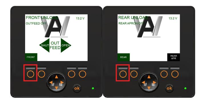
For combination (front/rear) unload units the first step couldn't be easier compared to other forage box systems. To select your unload method (front/rear) simply press the button noted above to switch between front and rear unload.
