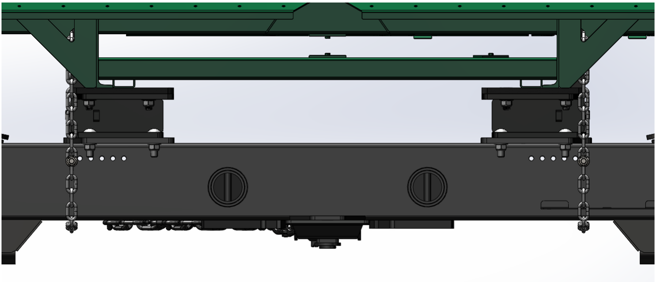
Horst 205 rear lashing as seen from rear of forage box.
