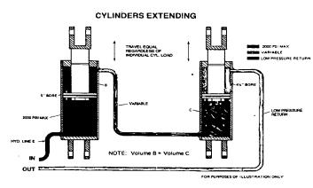
The lift cylinders are automatically kept in balance. External by-pass automatically allows oil to flow to lifting cylinder when piston reaches the end of its stroke in the retracting position.
