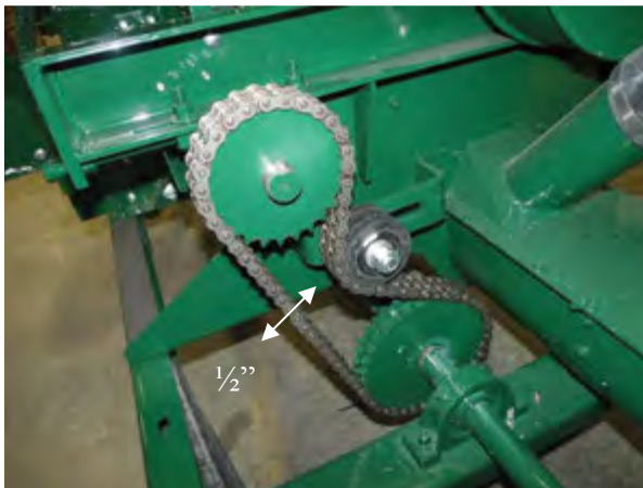
Figure 35 - Drive Chain Adjustment (Shields Removed for Clarity).
