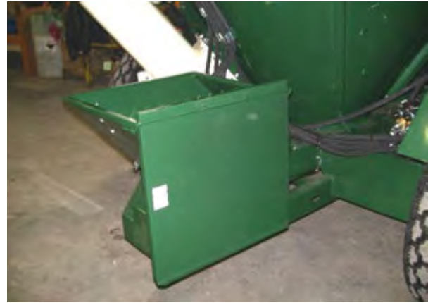
Figure 21 - Supplement Hopper Located on Center Rear Right Hand Side of Machine.
