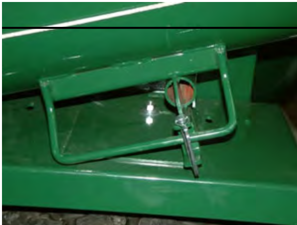
Figure 28 - Auger Feeder Latch Handle (Shown in Locked Position).
