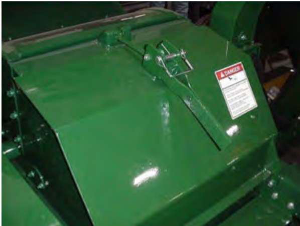
Figure 20 - Locking Pin and Latch on Hammer mill Door.
