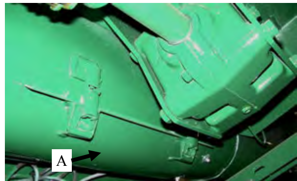
Figure 22 - Cleanout Door (A) Located Under Right Hand Side Of Tank Assembly.
