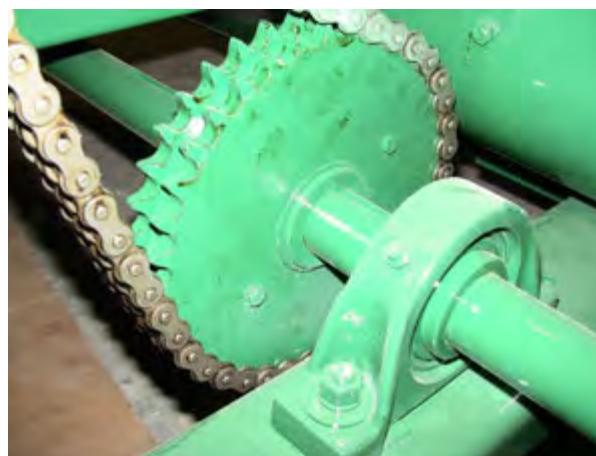
Figure 62 - Mixer Sprocket (Shields Removed For Clarity).
