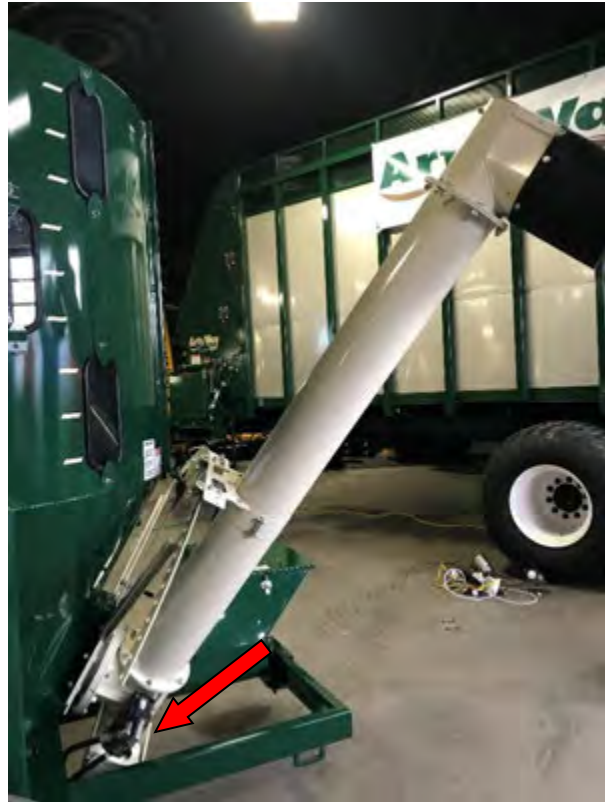
Figure 41 - Discharge Auger Drive Chain (See Arrows).
