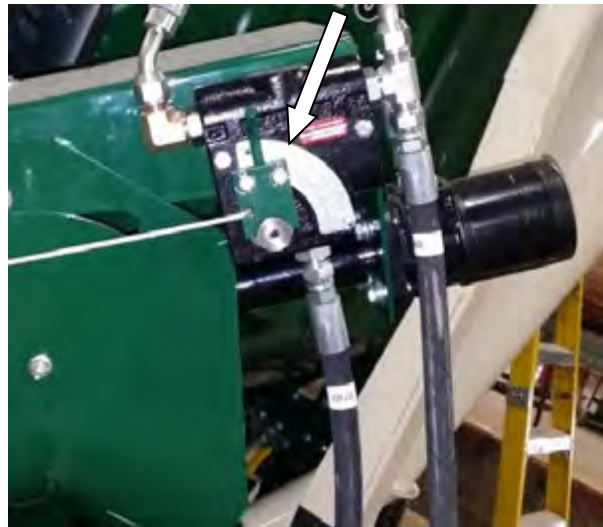
Figure 33 - Hydraulic Auger Feeder Control (Shown in Full Off Position) (See Arrow).
