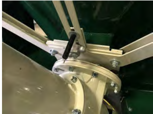
Figure 26 - Discharge Gate in closed position.
