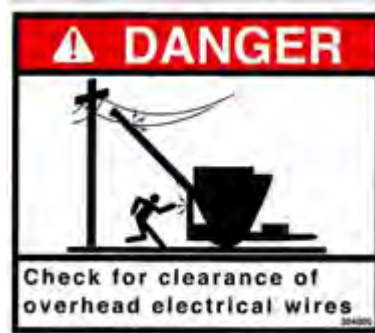
6. DANGER – Electrocutation Hazard (384000)
