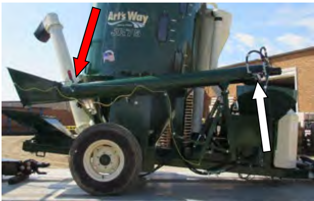
Figure 32 - Hydraulic Auger Feeder Controls (Shown in Off and Transport Position): Throttle Controls (White Arrow) and Emergency Shutoff (Red Arrow).
