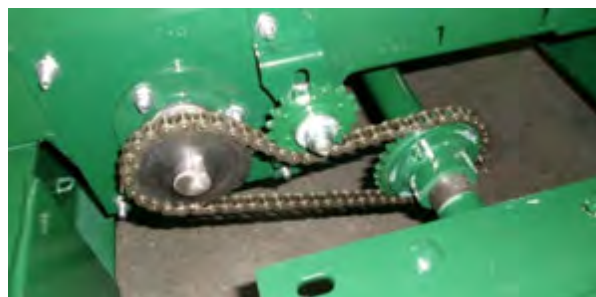
Figure 63 – Mill To Mixer Sprocket (Shields Removed For Clarity).
