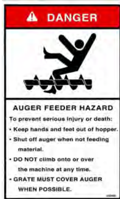
4. DANGER – Auger Feeder Hazard (383990)
