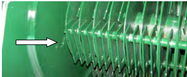
Figure 67 - Hammer Removal Hole To Remove Hammer Mill Rods (Shields Removed For Clarity).
