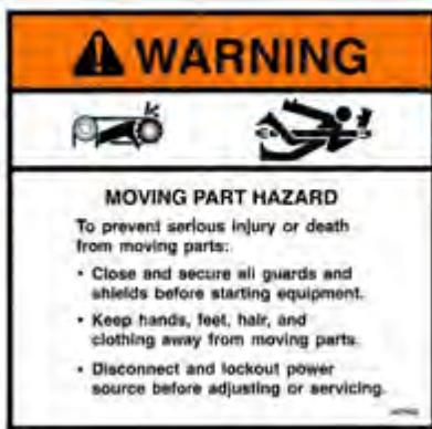
7. WARNING – Moving Part Hazard (467450)
