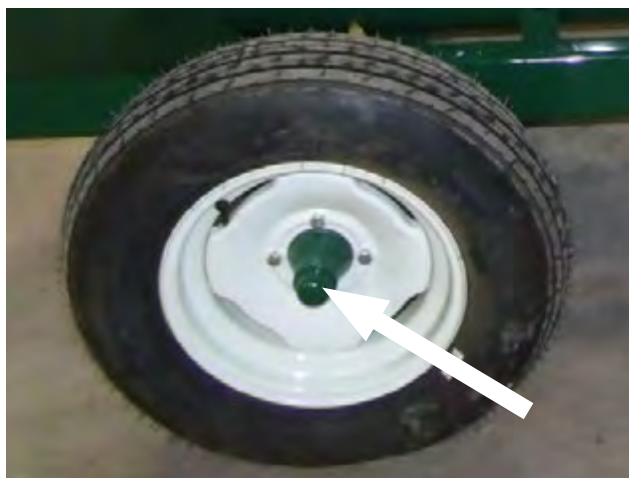
Figure 33 - Wheel Bearing Lubrication
