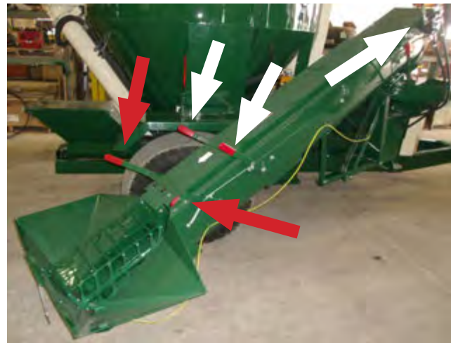
Figure 16 - Hydraulic Auger Feeder controls (shown in off position): Throttle controls (white arrows) and Emergency Shutoff (red arrows)
