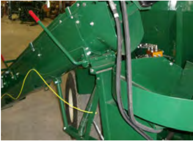
Figure 13 - Auger Feeder Positioner And Spring Adjustment
