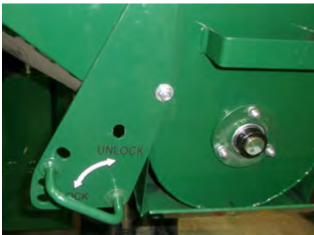
Figure 10 - Auger Feeder Latch Handle (Shown Locked)
