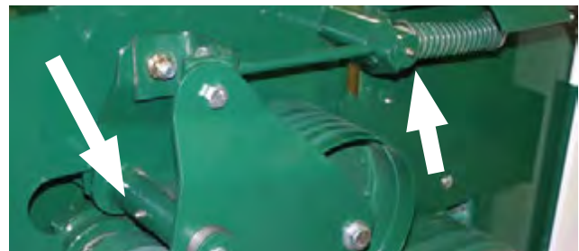
Figure 28 - Drive Belt Idler Tensioner
