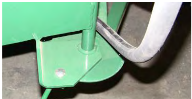
Figure 12 - Auger Feeder Swing Brake
