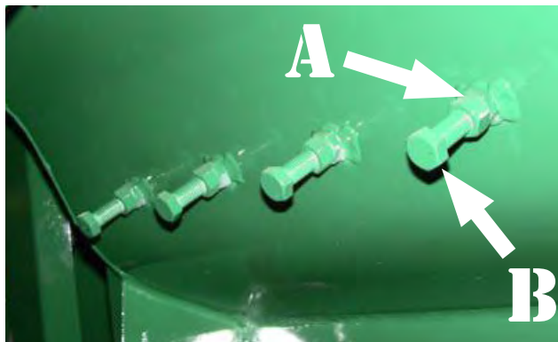
Figure 5 - Hay Retard Bolts (A - Lock Nut; B - Adjustable Retard Bolt, 26 Inch Hammer mill Shown)
