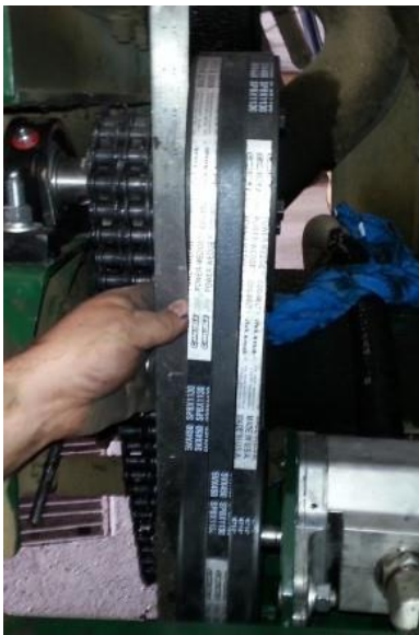
Figure 109a – Sheave Alignment (Use a Straight Edge).
