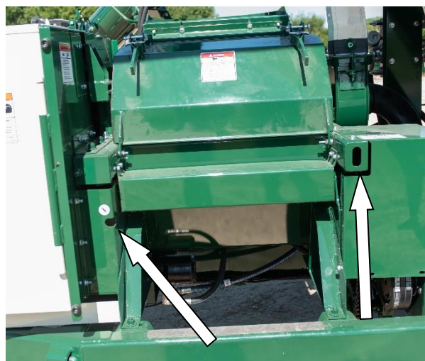
Figure 70 - Jack Shaft Front and Rear Bearings.
