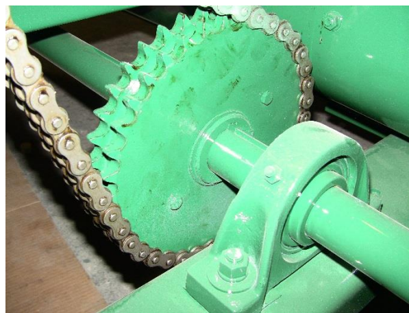
Figure 83 - Mixer Sprocket (Shields Removed for Clarity).
