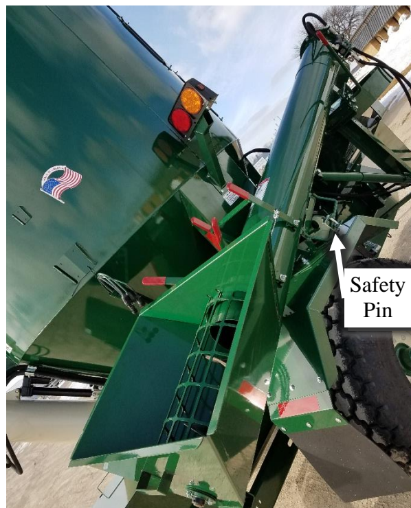
Figure 37 – Auger Feeder (Shown in Transport Position).
