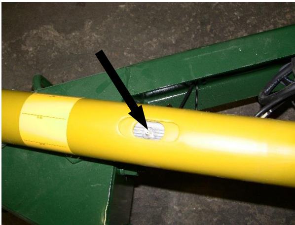
Figure 63 - PTO Driveline Shaft (See Arrow).
