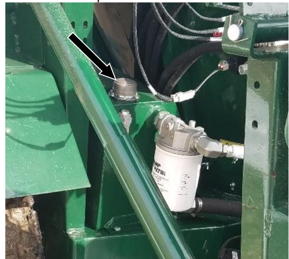
Figure 113a – Hydraulic Reservoir Cap (see Arrow)
