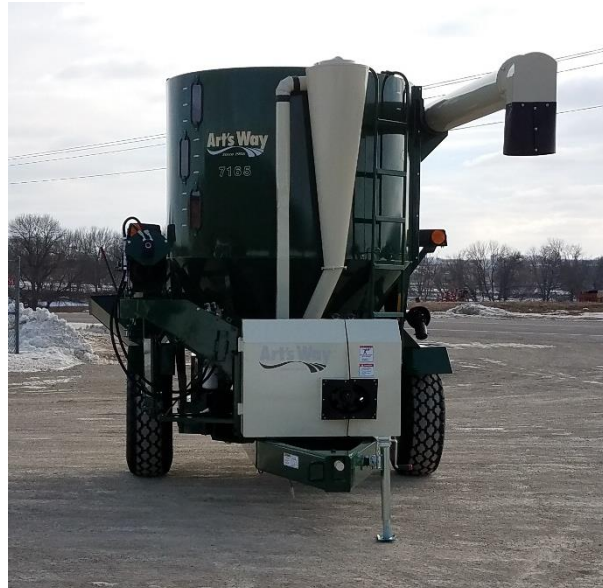
Figure 5 - Model 7165 With Self-Contained Hydraulics and Auger Feeder.
