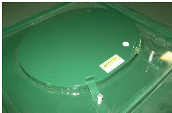
Figure 27 - Spring Loaded Tank Lid.
