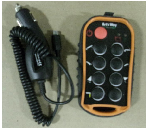
Figure 102 – Macro-Remote Control device with Charger.
