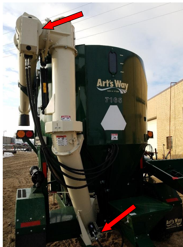
Figure 56 - Discharge Auger Drive Chain Locations (See Arrows).
