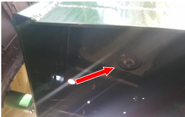
Figure 112 –Drain Underneath Reservoir Tank Base (Red Arrow).
