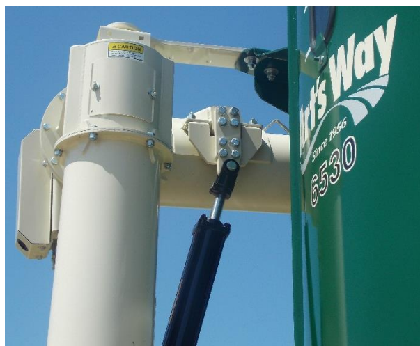
Figure 28 - Unloading Auger Positioning (Shown in Upper 60° to -11° Configuration).
