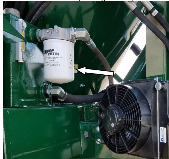
Figure 110 – Reservoir Filter (see Arrow)
