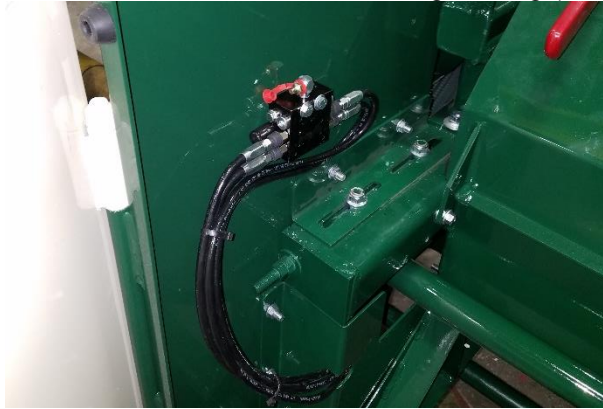
Figure 92, Detail B). Then relieve the belt tension by loosening the bolt (see Figure 92, Detail A) and move bearing mount and sheave.
