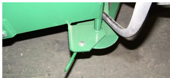
Figure 35 - Auger Feeder Swing Brake.
