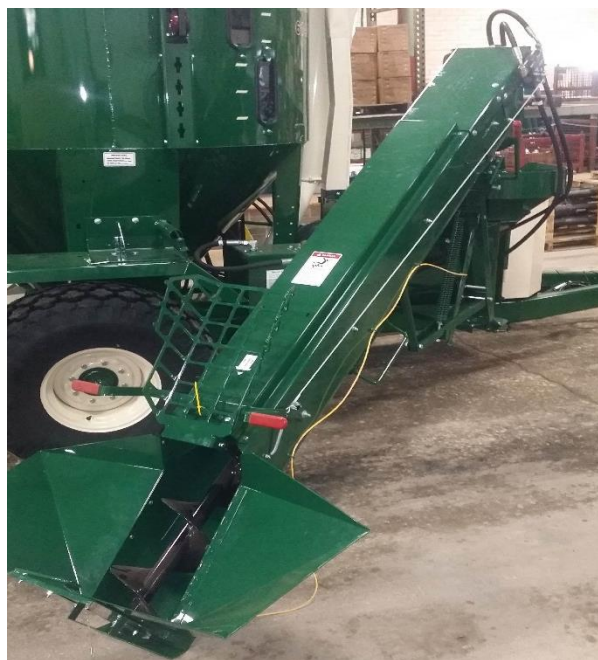
Figure 34 - Auger Feeder Operation (Grate in Lifted Position).
