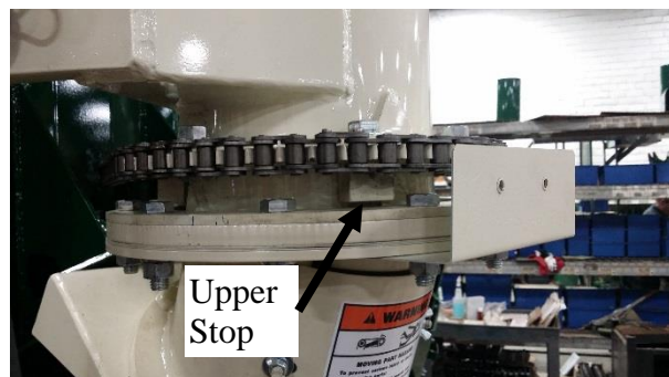
Figure 50 - Rear Swivel Stop (Shields Removed for Clarity).
