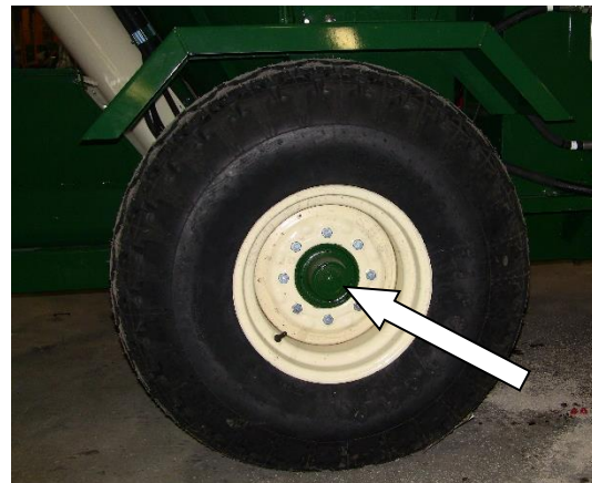
Figure 73 - Wheel Bearing Lubrication.
