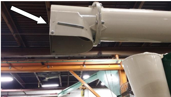
Figure 32 - Unloading Auger Hood.
