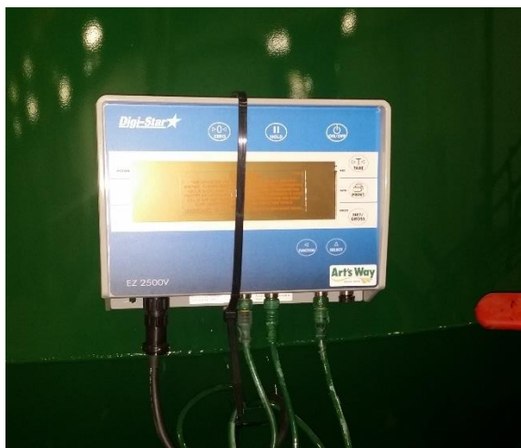
Figure 91 - Scale Head Attachment (EZ2500V Shown).
