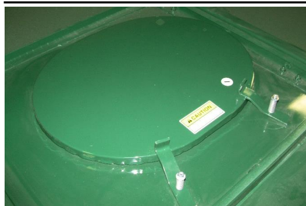
Figure 25 - Spring Loaded Tank Lid.
