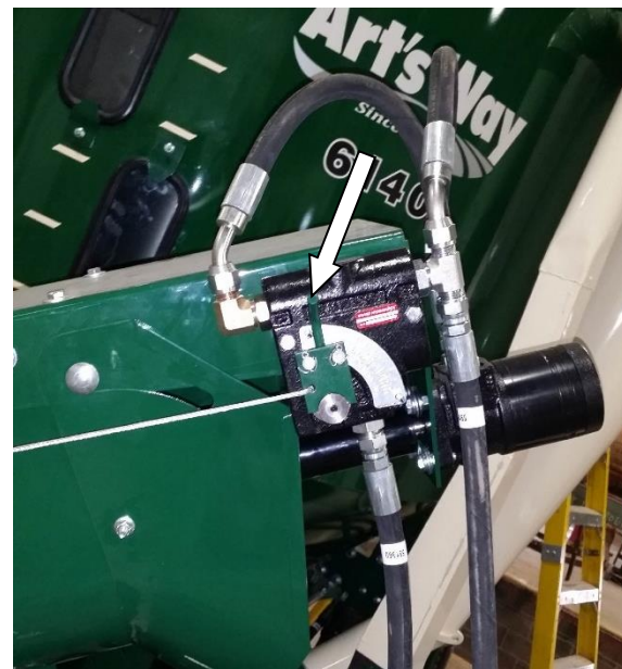
Figure 40 - Hydraulic Auger Feeder Control (Shown in Full Off Position) (See Arrow).
