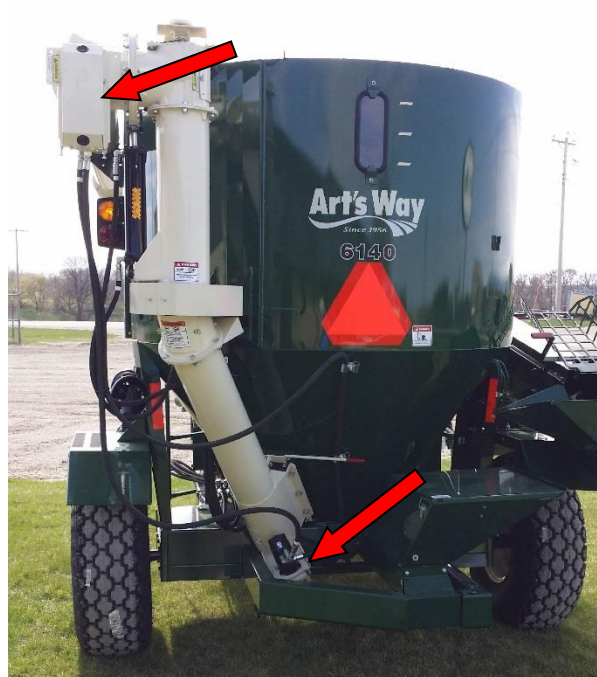
Figure 51 - Discharge Auger Drive Chain (See Arrows).
