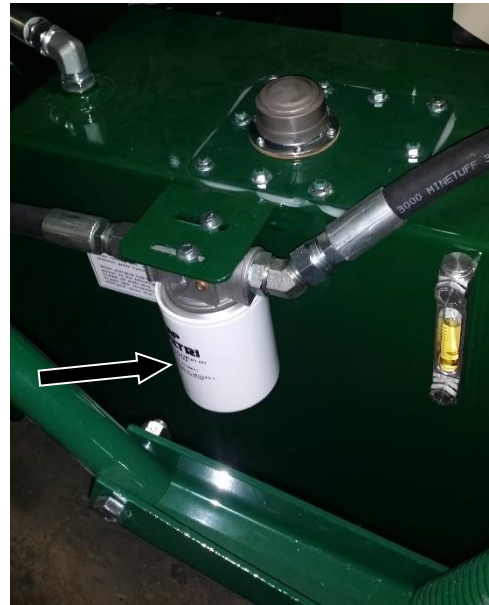
Figure 88 – Reservoir Filter (See Arrow).
