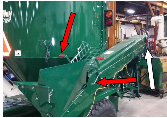
Figure 39 - Hydraulic Auger Feeder Controls (Shown in Off and Transport Position): Throttle Controls (White Arrow) and Emergency Shutoff (Red Arrows).
