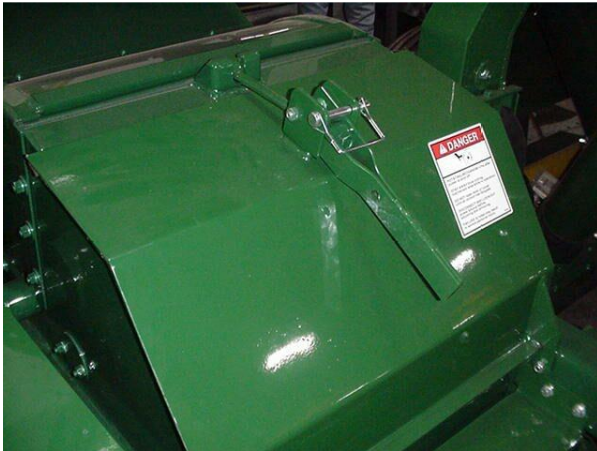
Figure 21 - Locking Pin and Latch on Hammer mill Door.
