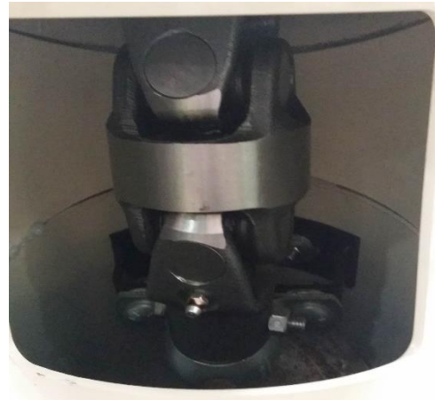
Figure 71 – Discharge U-Joint (Door Removed for Clarity).
