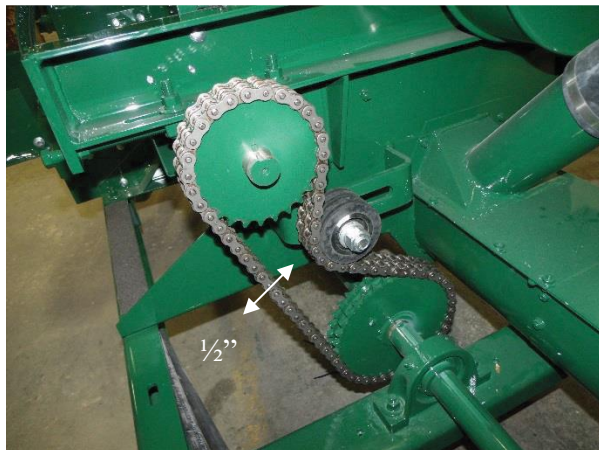
Figure 42 - Drive Chain Adjustment (Shields Removed for Clarity).
