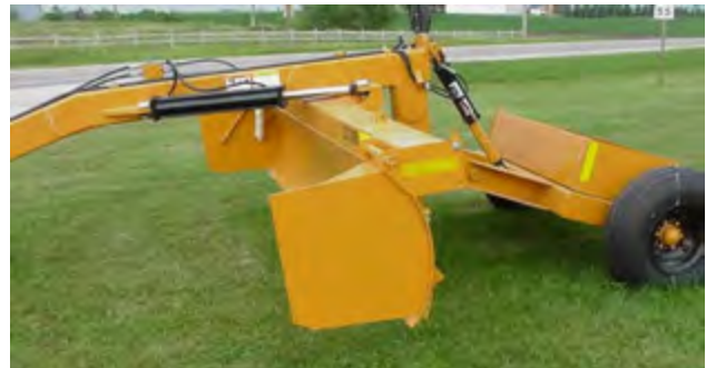
Figure 3. Box ends locked in down position.
