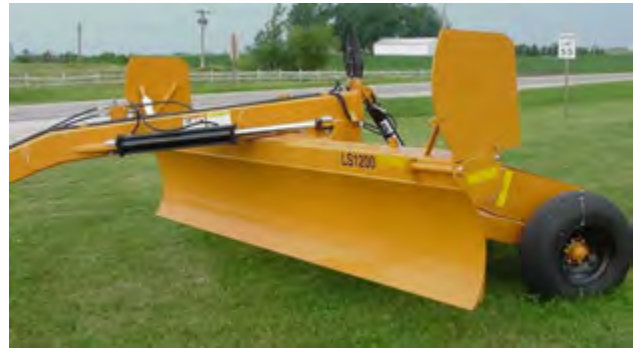
Figure 2. Box ends locked in up position.
