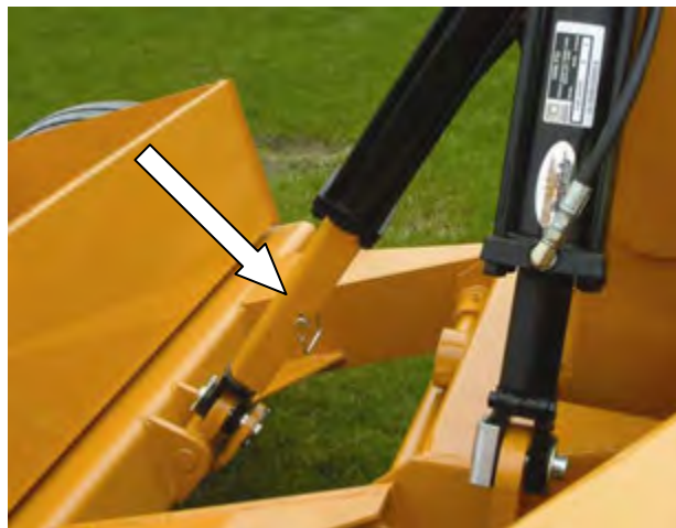
Figure 5. Lift cylinder mechanical safety stop.
