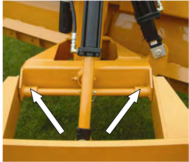
Figure 8. Lift pivot zerks (2).
