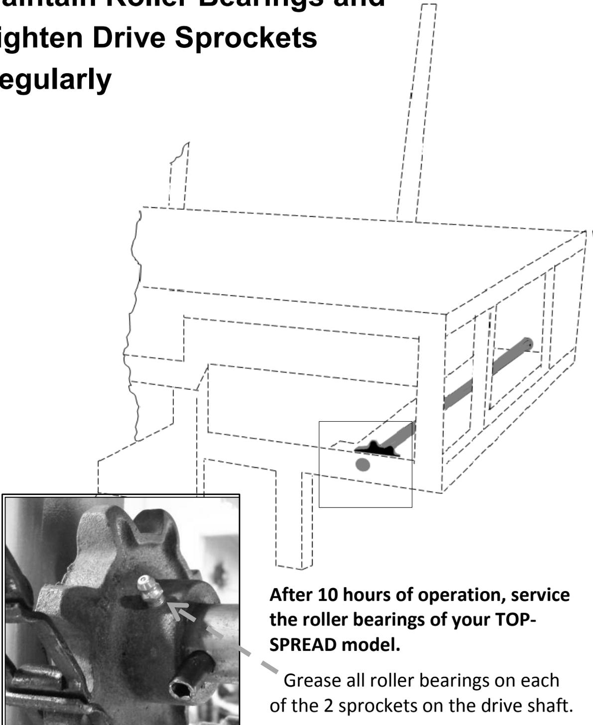
**After 10 hours of operation, service the roller bearings of your TOP-SPREAD model.**
