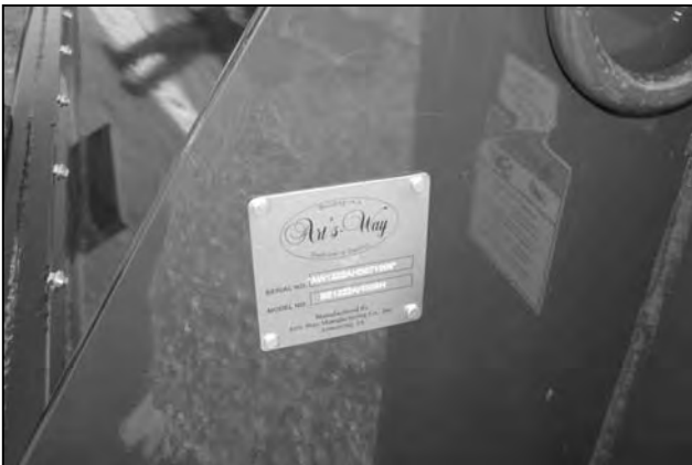
Figure 1 - Location of Serial & Model Number Placard on Defoliator
