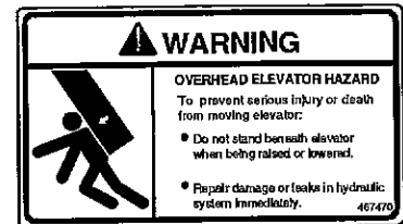
H - "WARNING" - Overhead Elevator Hazard. Part No. 467470
