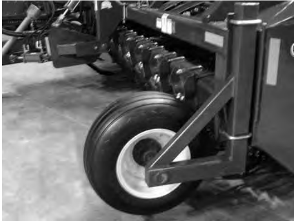
Figure 63 - Front Head Gage Wheels (Standard on 8 row 28/30, 9 row 24/26, and 12 row 22 Heads - Optional on 6 row 22/24, 6 row 28/30, and 8 row 22 Heads)
