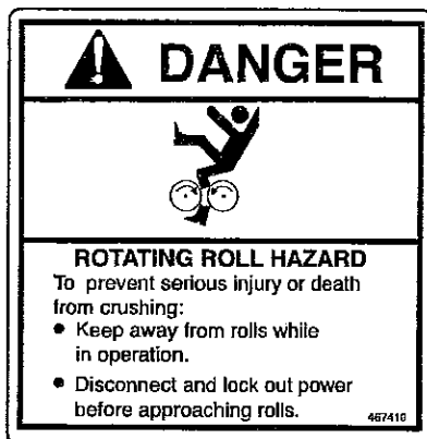
3 - "DANGER" - Rotating Roll Hazard. Part No. 467410
