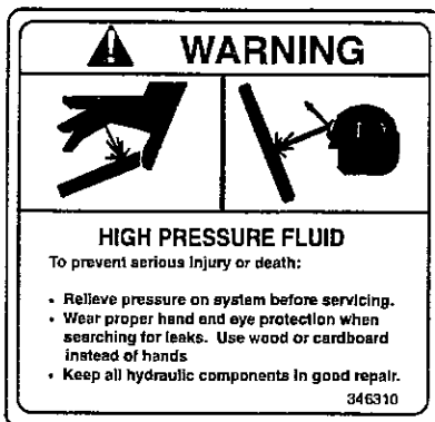
6 - "WARNING" - High Pressure Fluid. Part No. 346310
