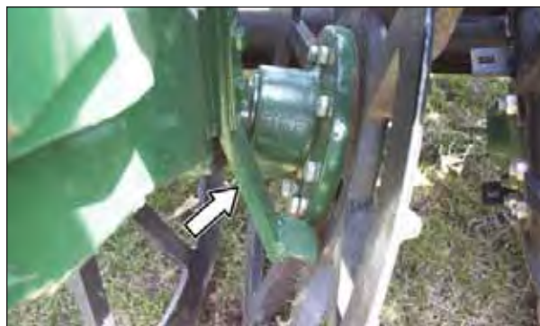
Figure 28. – Lifter Wheel Scrapers
