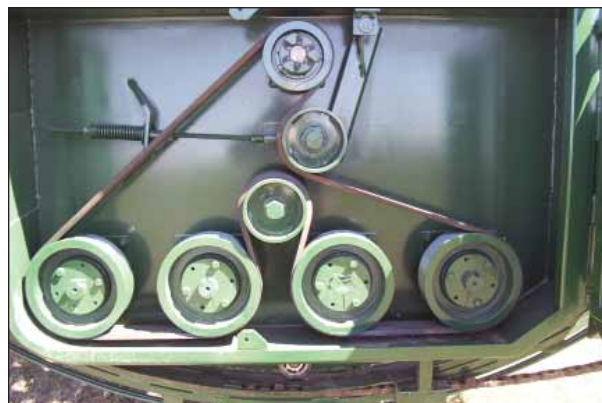
Figure 37. – Harvester Rear Belt Drive System
