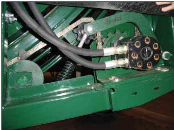
Figure 40. – Wheel Elevator Hydraulic Motor, Sprocket, Chain Drive, and Roller
