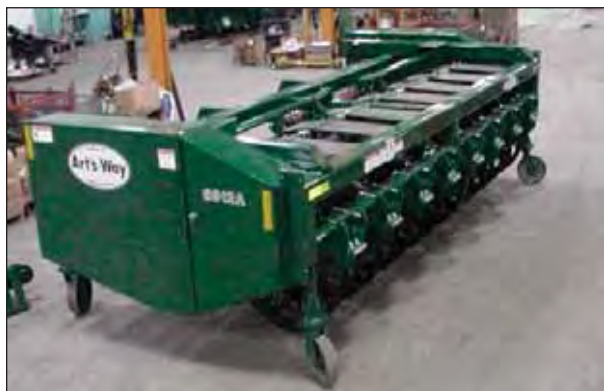
Figure 26. – Header (8 Row - 22 inch Header Shown)
