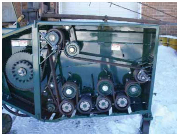
Figure 33. – Header Left-Hand Drive With Diverter Grab Roll Option (12 Row 22 And 8 Row 30)
