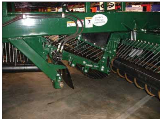
Figure 20. – Draper Chain Drives, Short Conveyor Shown
