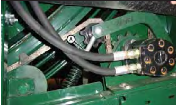
Figure 71. – Wheel Elevator Sprocket, Chain Drive, and Roller
