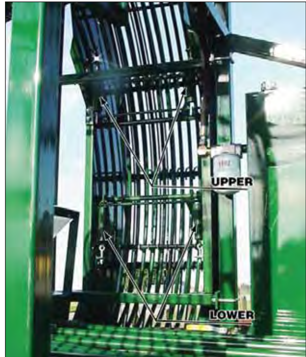
Figure 72. – Wheel Elevator Retainer Springs
