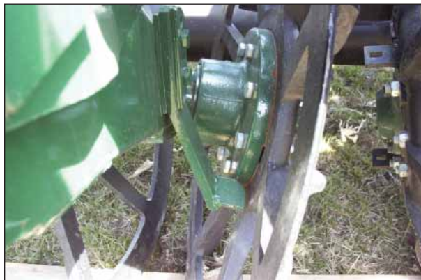
Figure 54. – Header Lifter Wheel Scraper Adjustments
