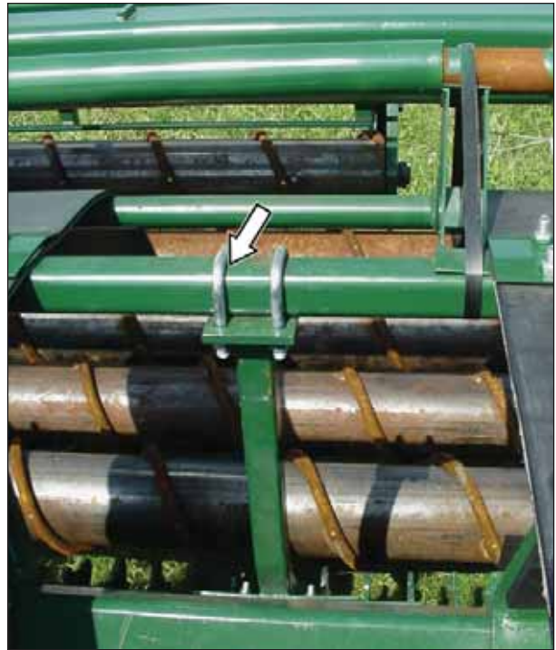
Figure 57. – Barrier U-Bolts (Used on all but the center barrier)
