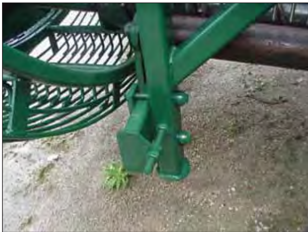
Figure 68. – Harvester Grabrollers - Single Point Adjustment (Back)
