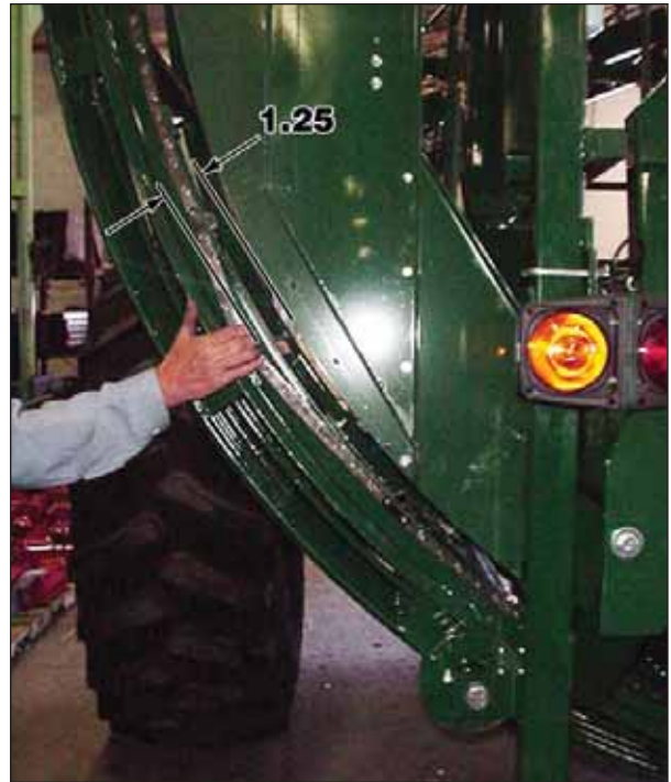
Figure 69. – Tension of Wheel Drive Chain
