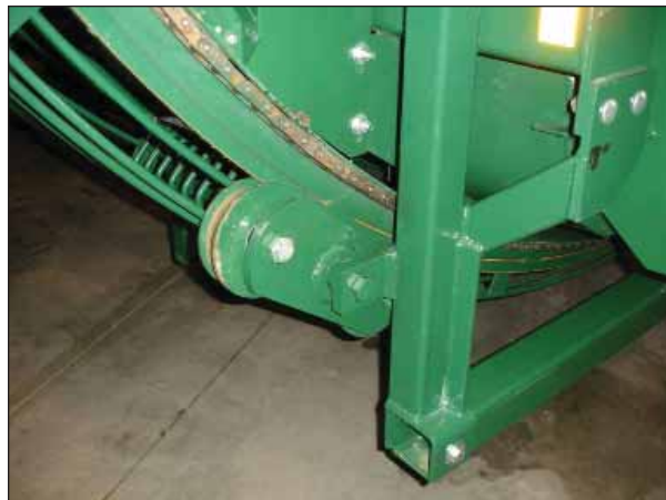
Figure 41. – Wheel Elevator Roller (Left-Hand Side)
