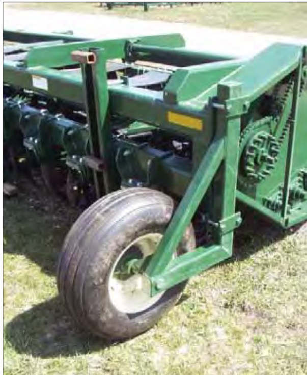
Figure 63. – Front Head Gage Wheels (Standard on 8 row 28/30, 9 row 24/26, and 12 row 22 Heads - Optional on 6 row 22/24, 6 row 28/30, and 8 row 22 Heads)
