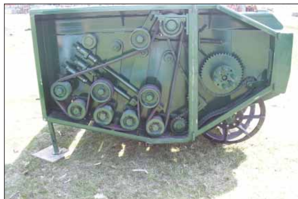
Figure 82. – Header Left-Hand Drive. (8 Row Header Shown)
