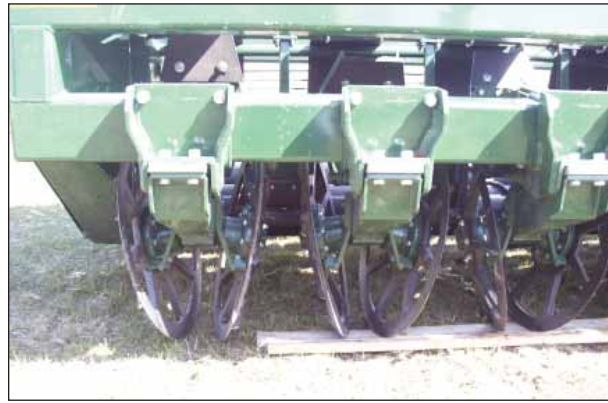
Figure 51. – Header Lifter Wheel Lateral Adjustment
