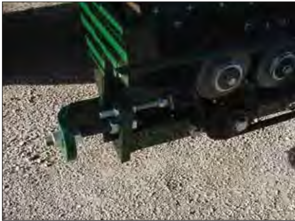
Figure 67. – Harvester Grabrollers - Single Point Adjustment (Front)
