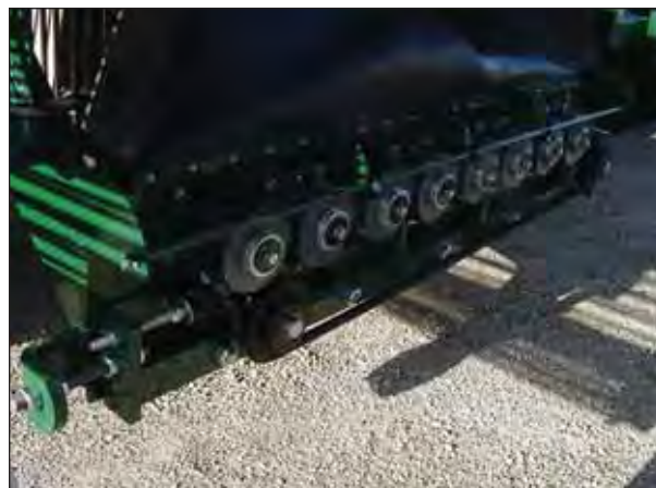
Figure 38. – Harvester Grab Rollers Front Drive
