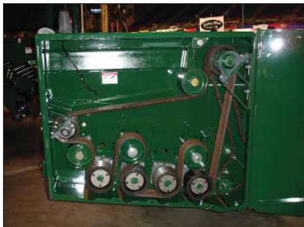
Figure 13. – Harvester Right-Hand Belt Drive (Rear Grabroll Option Shown)
