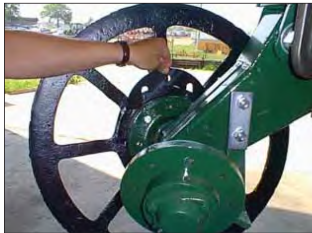
Figure 52. – Header Lifter Wheel Width Shims
