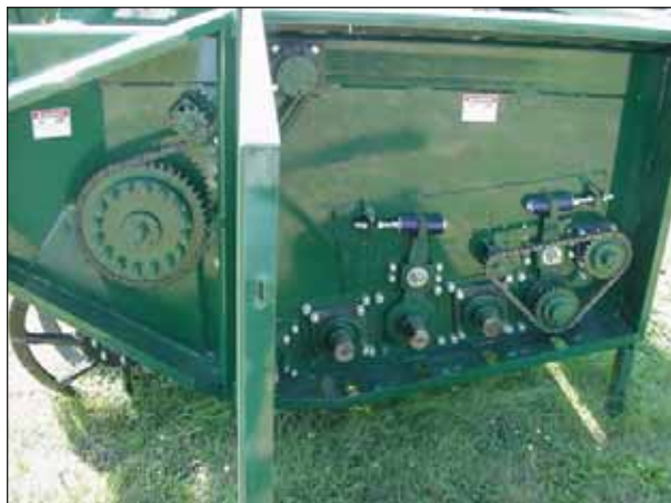
Figure 32. – Header Left-Hand Drive. (8 Row 22 Header Shown)
