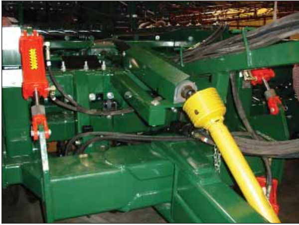
Figure 9. – Hydraulic Connection, Needle Valve Near The Front Left Corner
