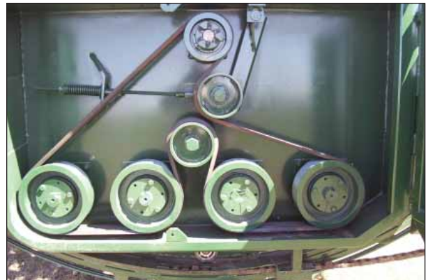
Figure 15. – Harvester Rear Belt Drive System and Pump Drive
