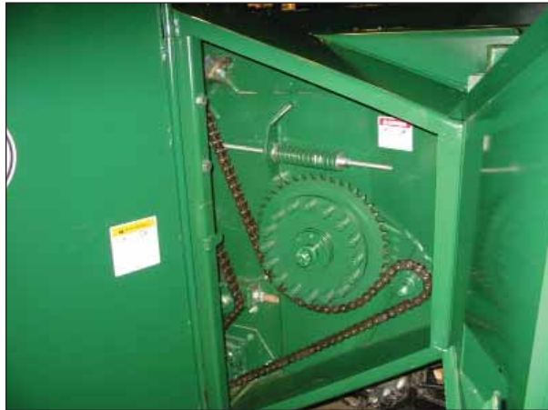
Figure 12. – Header Left-Hand Paddle Shaft Chain/ Drive
