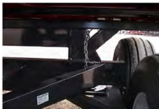
Figure 23 - Rear Saddle Tie Down Chains (LH)
