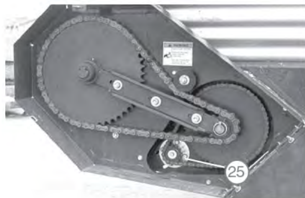
Figure 54 - Hydraulic Drive Chain (Rear Unload)
