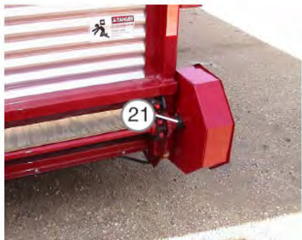
Figure 44 - Sprocket Bearing (Rear Unload Mechanical Drive Only - 1 Location)
