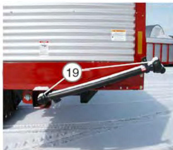
Figure 42 - Driveline Joints (Rear Unload Mechanical Drive Only - 2 Locations)
