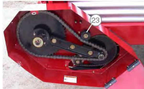
Figure 52 - Apron Drive Chain (Rear Unload)
