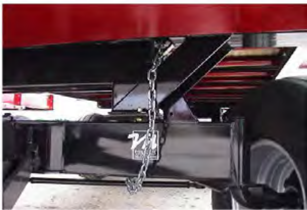
Figure 21 - Front Saddle Tie Down Chains (LH)
