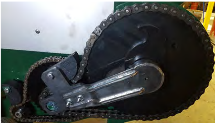
REAR SPROCKET SHOWN WITH NUT, LUG, AND BOLT REMOVED.
