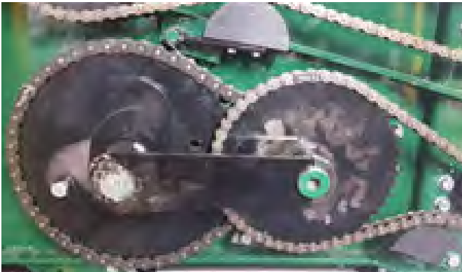
FRONT SPROCKET SHOWN WITH NUT, LUG, AND BOLT INSTALLED.
