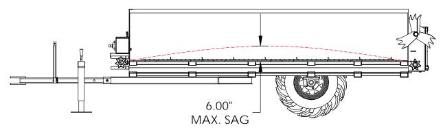
Grab apron in the center and pull up. There should be no more than 6" of sag. If apron is loose, remove one link from each side of that apron chain assembly and readjust to tension as shown. **CAUTION:** Over tightening can cause premature failure of the drive components.
