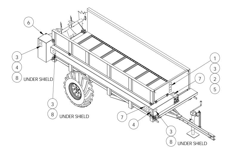
**MODEL AND SERIAL NUMBER INFORMATION** is located in the upper center area of the front panel. This is the number to give service personnel for parts and service questions.
