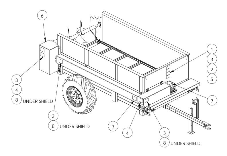
**MODEL AND SERIAL NUMBER INFORMATION** is located in the upper center area of the front panel. This is the number to give service personnel for parts and service questions.
