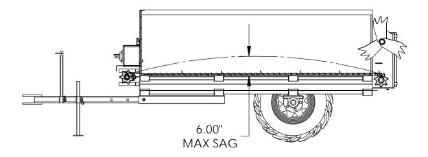
Grab apron in the center and pull up. There should be no more than 6" of sag. If apron is loose, remove one link from each side of that apron chain assembly and readjust to tension as shown. **CAUTION:** Over tightening can cause premature failure of the drive components.
