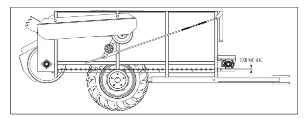
If apron is loose, remove one link from each side of that apron chain assembly and readjust to tension as shown. **CAUTION:** Over tightening can cause premature failure of the drive components.
