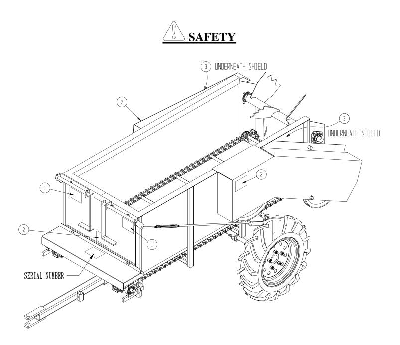
**MODEL AND SERIAL NUMBER INFORMATION** is located in the upper center area of the front apron shield. This is the number to give service personnel for parts and service questions.
