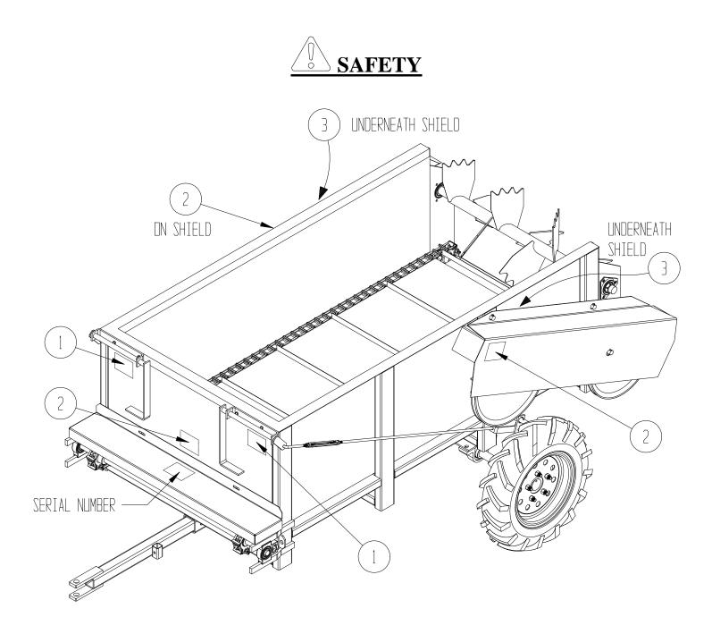
**MODEL AND SERIAL NUMBER INFORMATION** is located in the upper center area of the front apron shield. This is the number to give service personnel for parts and service questions.
