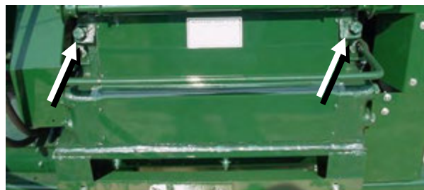
Figure 11 - Grain Control Gate Lubrication (2 Zerks And Slide Guides).
