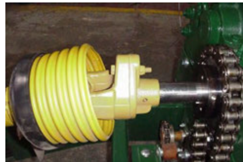
Figure 4 - PTO Driveline Shear Clutch
