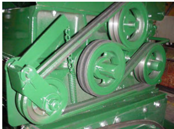
Figure 8 - Belt Adjustment (Shields Removed For Clarity).
