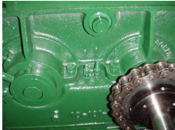
Figure 7 - Roll Scraper Adjustment Bolts
