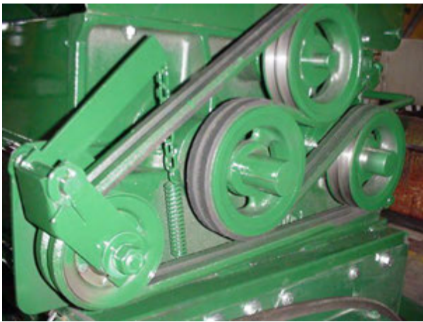
Figure 13 – Roller mill Belt Drive
