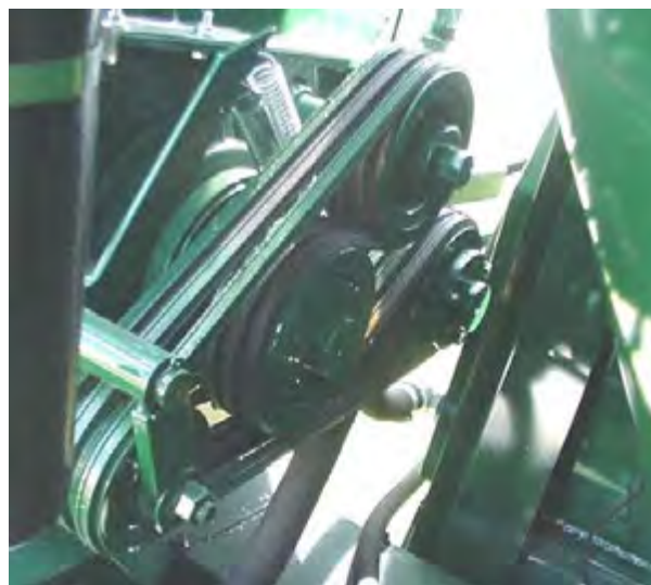
Figure 63 – Roller mill Belt Drive (shield removed for clarity).
