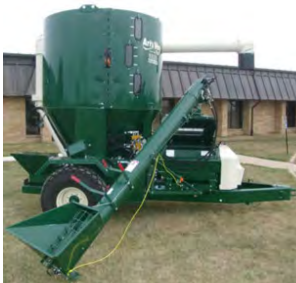
Figure 8 - Model 6530 CattleMaxx With Self-Contained Hydraulics, Auger Feeder.
