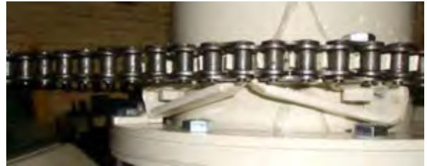
Figure 50 - Hydraulic Swing Adjustment (Shields Removed For Clarity).
