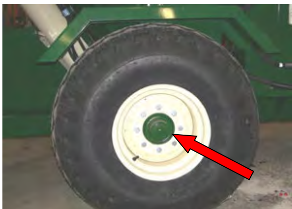
Figure 76 - Wheel Bearing Lubrication.
