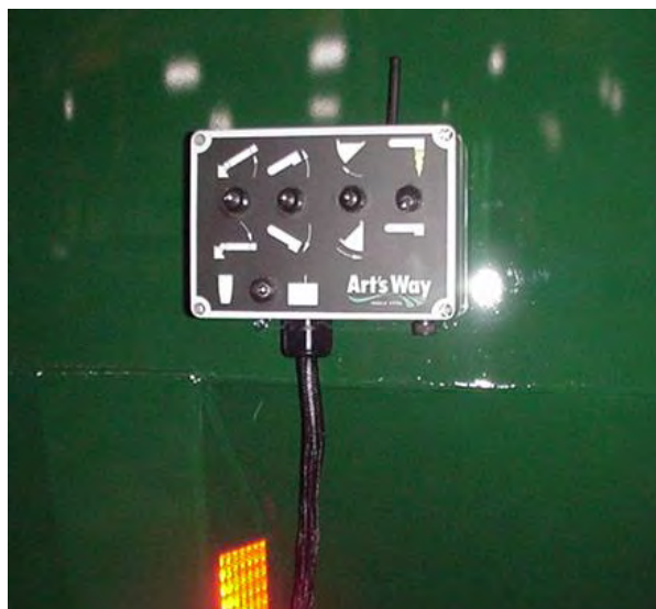
Figure 85 – Complete Control Box with internal Receiver as Backup Remote Control Box mounted on left rear side of mixer tank (for functions see Figure 90).
