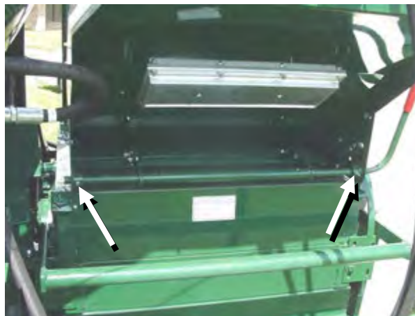
Figure 61 - Grain Control Gate Lubrication (2-Zerks and Slide Guides).
