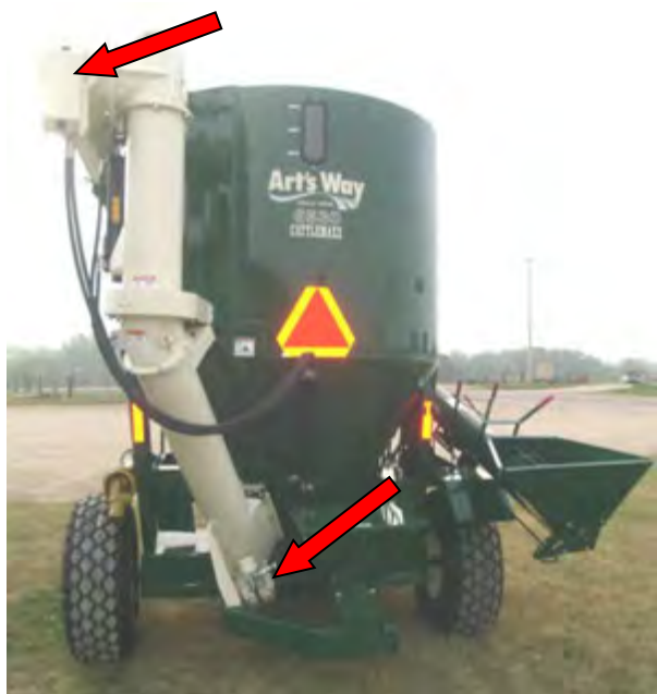
Figure 52 – Discharge Auger Drive Chain Locations (see arrows).
