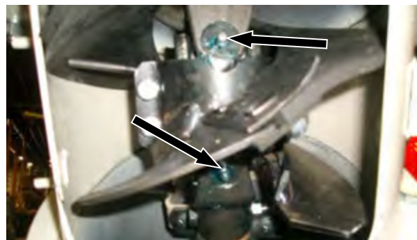
Figure 74 – Discharge U-Joint (Door Open for Clarity).
