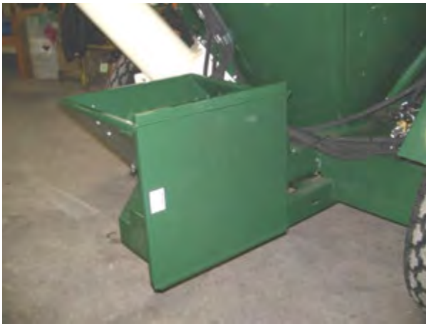
Figure 22 - Supplement hopper located on center rear right hand side of machine
