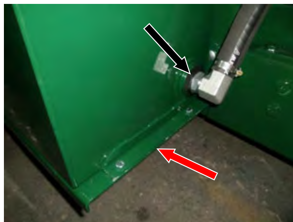
Figure 97 – Reservoir Strainer (black arrow) and Drain underneath reservoir tank base (red arrow).
