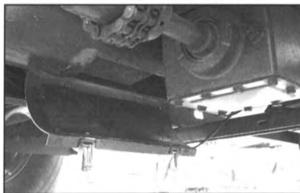
Figure 22 - Clean-Out Door Located Under Right-Hand Side Of Tank Assembly.
