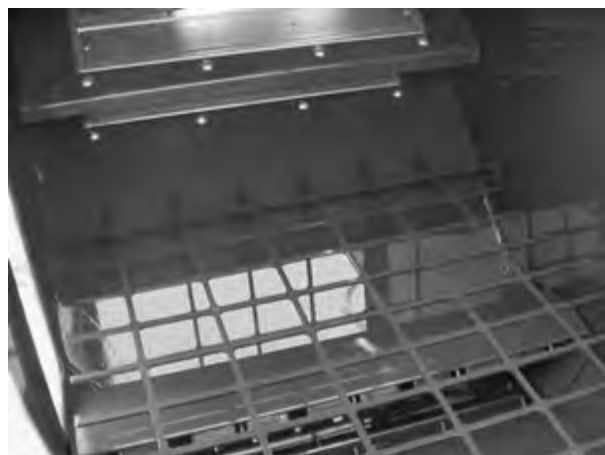
Figure 45 - Removing Magnet To Check Roll Spacing.
