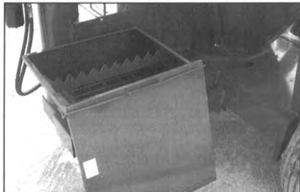
Figure 20 - Supplement Hopper On Right-Hand Side Of Machine.
