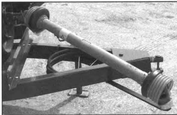
Figure 56 - PTO Driveline (Shield Removed For Clarity).
