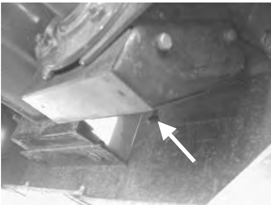
Figure 71 - Discharge Auger Bevel Gears, Outer Elbow (Shields Removed For Clarity).
