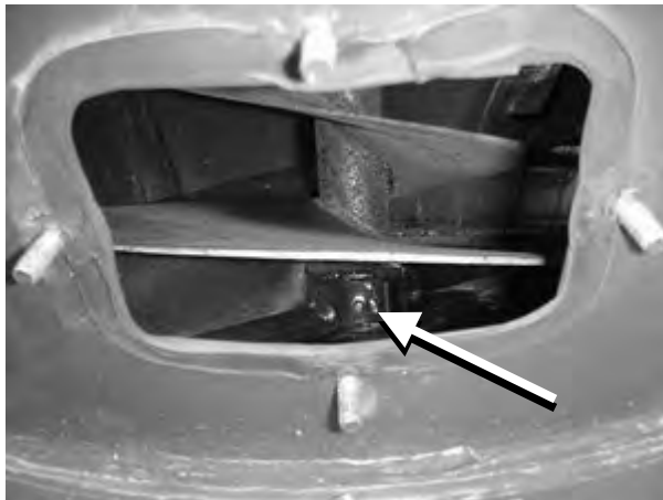
Figure 65 - Clean-Out Door in Mixing Tank Cone And Grease Zerk For Seal At Bottom Of Vertical Mixing Auger.
