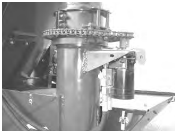
Figure 50 - Hydraulic Swing Adjustment (Shields Removed For Clarity).
