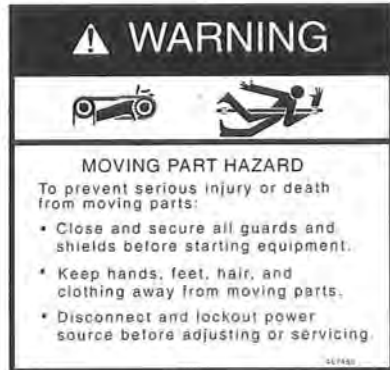
8. WARNING - Moving Part Hazard (384020)
