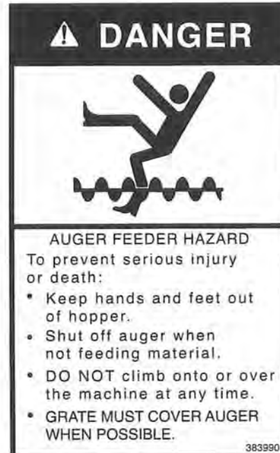
5. DANGER - Auger Feeder Hazard (383990)
