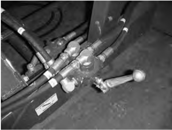
Figure 39 - Hydraulic Auger Feeder Selector Valve Lever Is In The Out Position - Auger Feeder).
