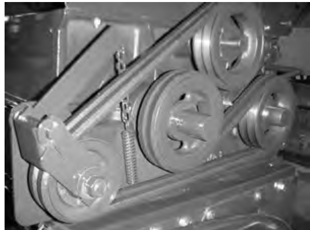
Figure 43 - Drive Chain Adjustment (Shields Removed For Clarity).
