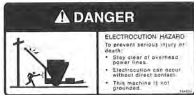
6. DANGER - Electrocution Hazard (384000)
