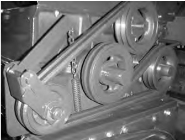
Figure 60 – Rollermill Belt Drive
