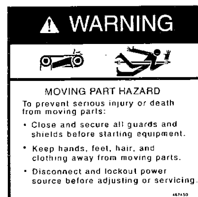
No. 8 - "Warning" - Moving part hazard. Part No. 467450.
