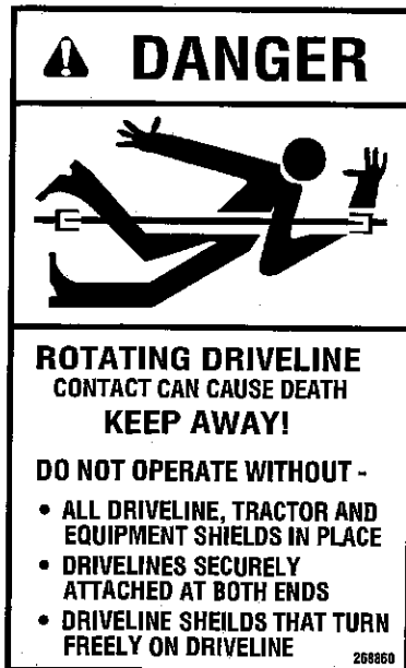
No. 2 - "Danger" - Rotating drive line (located on PTO). Part No. 268860.
