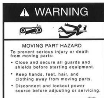
7. WARNING - Moving Part Hazard
