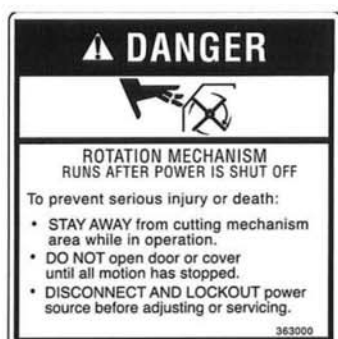
1. DANGER - Rotation Mechanism
