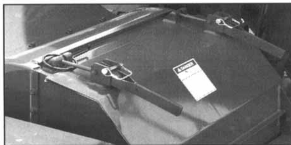
Figure 21 - Locking Pin And Latch On Hammermill Door (26 Inch Hammermill Shown).
