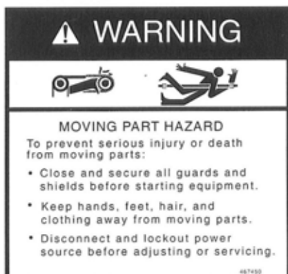
8. WARNING - Moving Part Hazard (384020)
