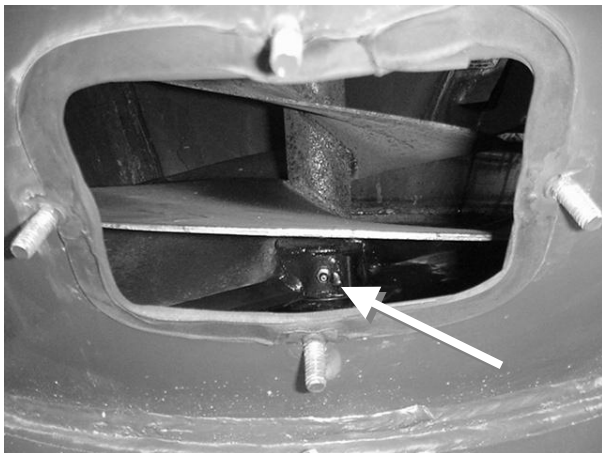
Figure 66 - Clean-Out Door in Mixing Tank Cone And Grease Zerk For Seal At Bottom Of Vertical Mixing Auger.
