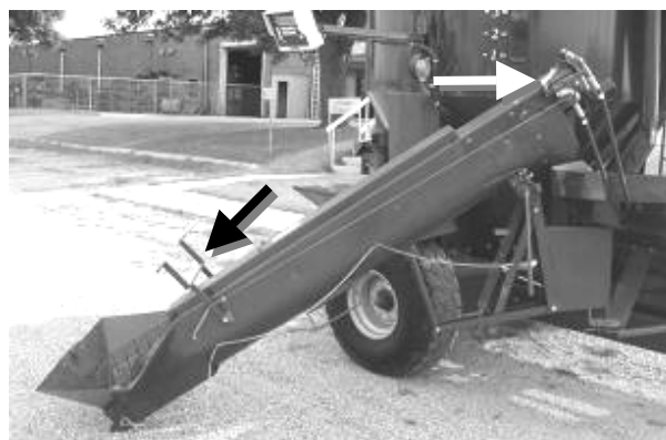
Figure 36 - Hydraulic auger feeder controls (See arrows.)
