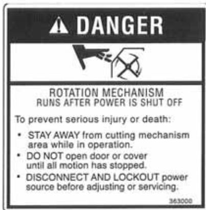
1. DANGER - Rotation Mechanism (363000)
