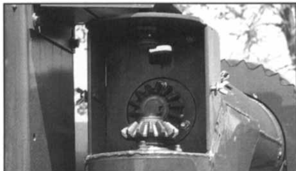
Figure 70 - Discharge Auger Bevel Gears, Inner Elbow (Shields Removed For Clarity).
