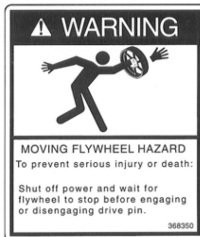
7. WARNING - Moving Flywheel Hazard (368350)
