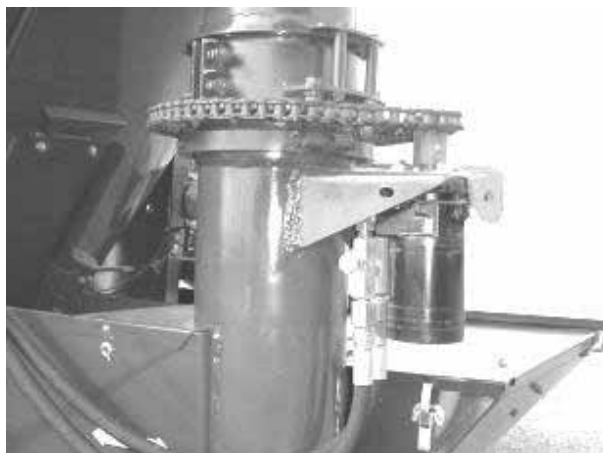
Figure 47 - Hydraulic Swing Adjustment (Shields Removed For Clarity).
