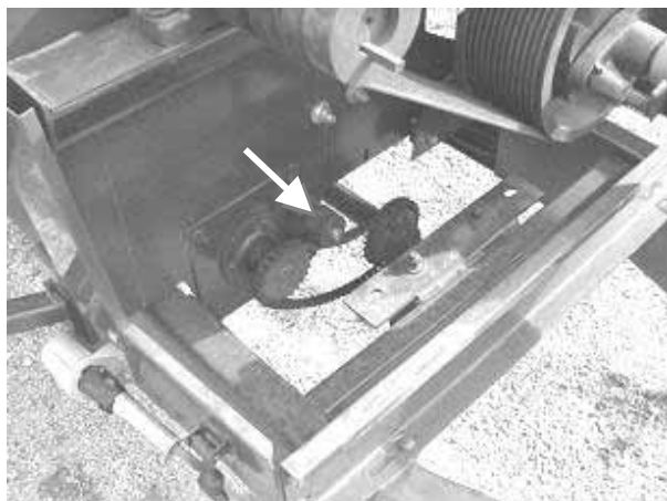
Figure 39 - Mill To Mixer Auger Drive Chain.
