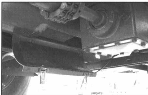
Figure 23 - Cleanout Door Located Under Right Hand Side Of Tank Assembly.
