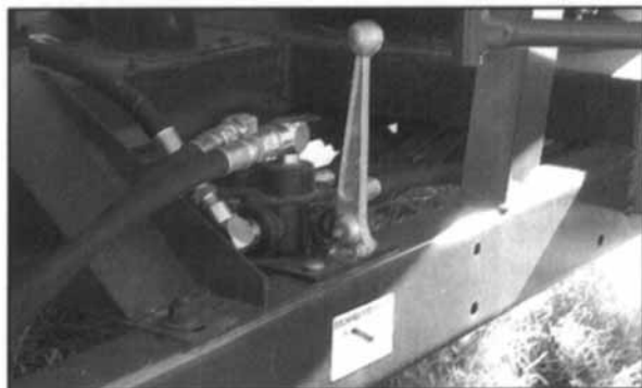
Figure 26 - Hydraulic Selector Valve (Lever In The In Position - Hydraulic Swing).
