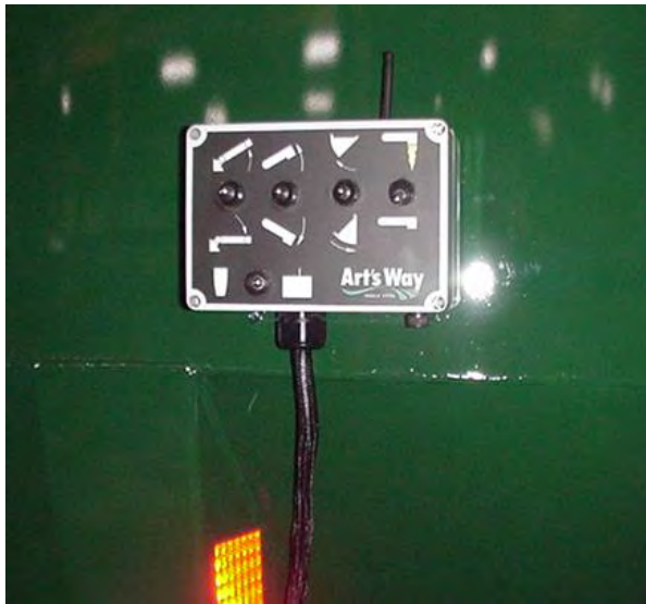
Figure 87 – Complete Control Box with internal Receiver as Backup Remote Control Box mounted on left rear side of mixer tank (for functions see Figure 90A).
