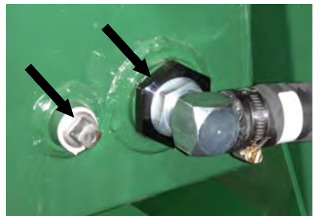
Figure 96 – Reservoir Strainer (on Right) and Drain (on Left)
