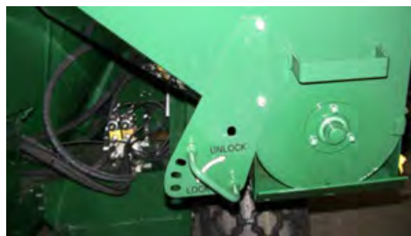
Figure 32 – Auger Feeder Latch Handle (shown in locked position).
