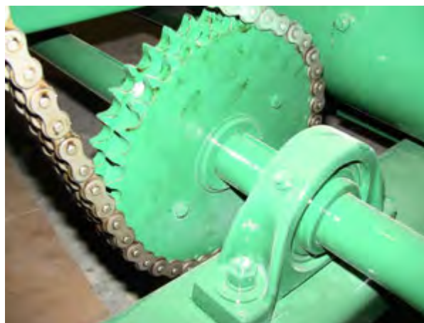
Figure 73 - Mixer Sprocket (Shields Removed For Clarity).
