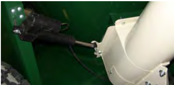
Figure 27 - Discharge Gate with Electric Actuator in closed position.
