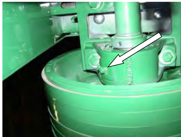
Figure 59 - Jack Shaft Front Bearing, Front (Looking Up Under Machine)
