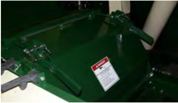
Figure 21 - Locking Pin and Latch on Hammer mill Door.
