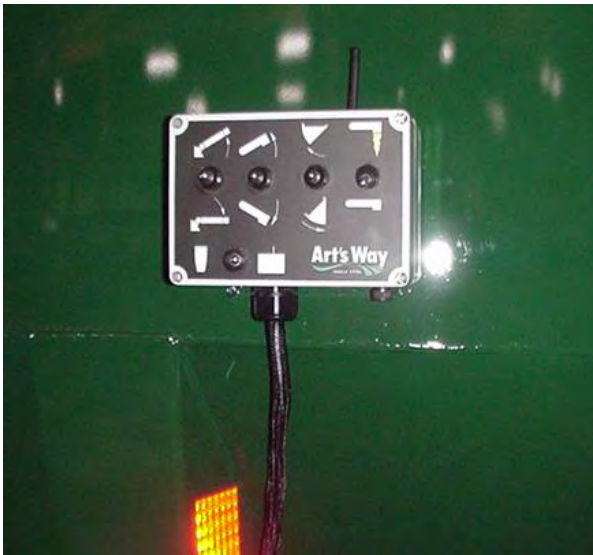
Figure 90 – Complete Control Box with internal Receiver mounted on left rear side of tank.
