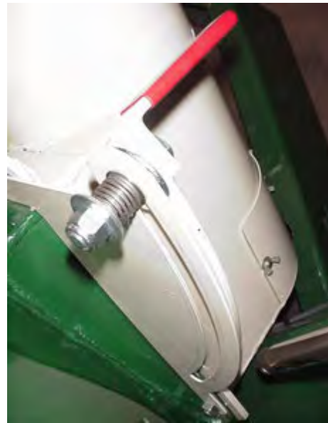
Figure 28 - Discharge Gate with Manual Handle in open position.
