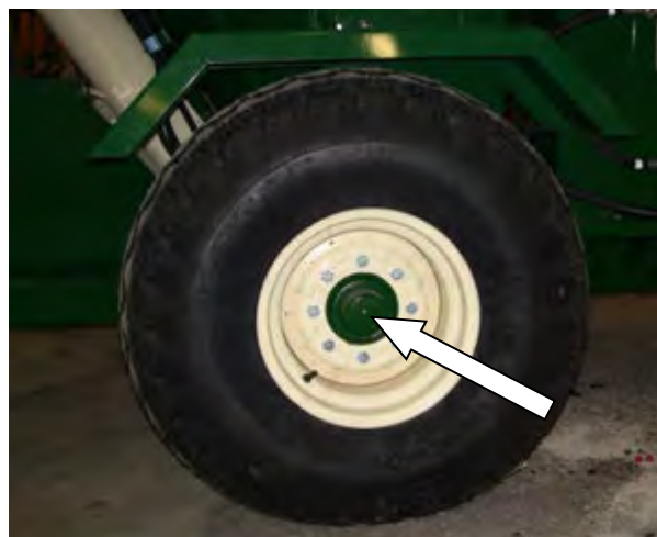
Figure 71 - Wheel Bearing Lubrication.
