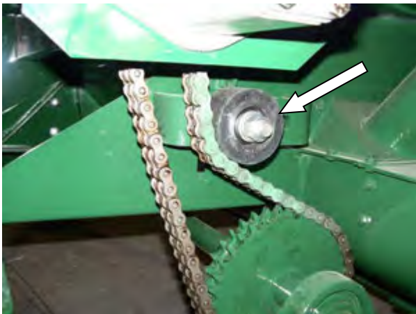
Figure 40 - Drive Chain Adjustment (Shield Removed for Clarity).
