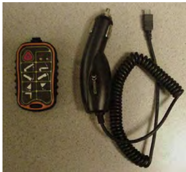
Figure 88A – Micro-Remote Control device with Charger (button functions same as Mini-Controller - Figure 88).
