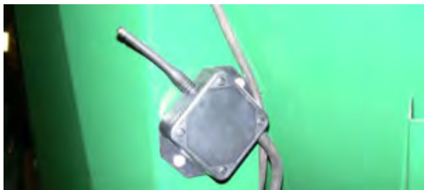
Figure 84 – Separate Receiver mounted on frame (early units).
