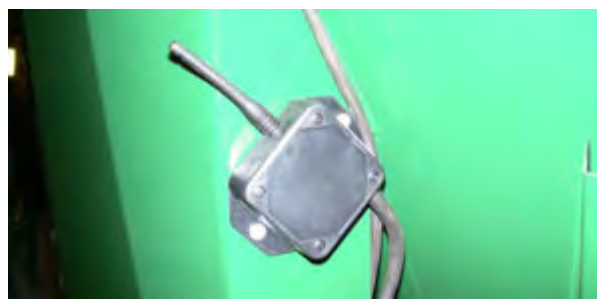
Figure 89 – Receiver (early units) mounted on right side of frame.
