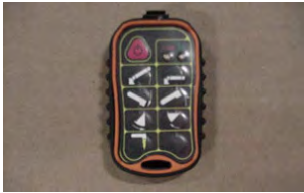
Figure 83A – Micro-Wireless Remote Control (buttons same as Mini-Controller).
