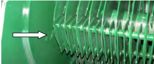
Figure 77 - Hammer Removal Inside Hammer mill, Hole to Remove Hammer mill Rods (Shields Removed For Clarity).
