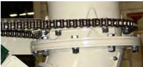
Figure 48 - Hydraulic Swing Adjustment (Shields Removed For Clarity).
