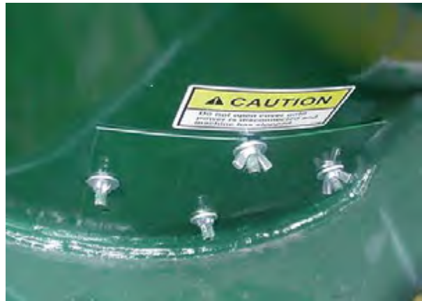
Figure 23 - Tank Cone Clean-Out Door (Left-Hand Side shown).
