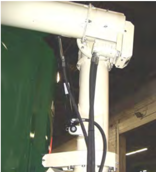
Figure 27 – Discharge Auger Positioning.
