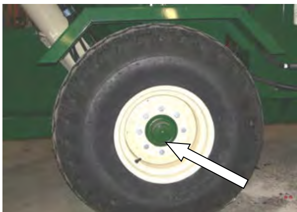
Figure 70 - Wheel Bearing Lubrication.
