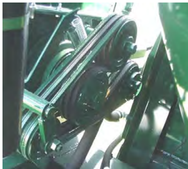
Figure 57 – Roller mill Belt Drive (shield removed for clarity).
