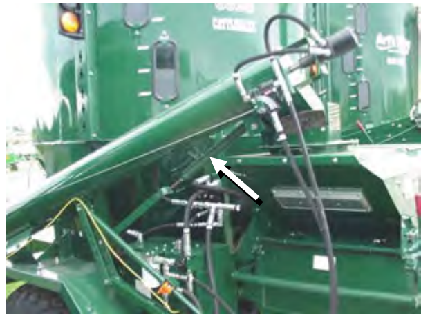
Figure 36 – Auger Feeder Counter Balance Spring
