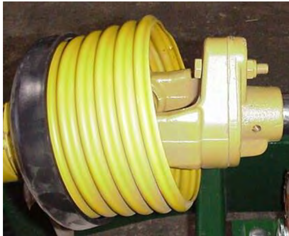
Figure 18 - PTO Driveline Shear Clutch
