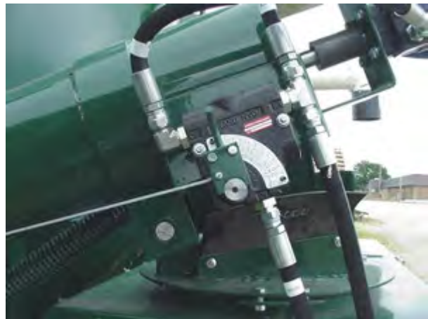
Figure 38 - Auger Feeder Flow Control Valve (Shown In "OFF" Position).
