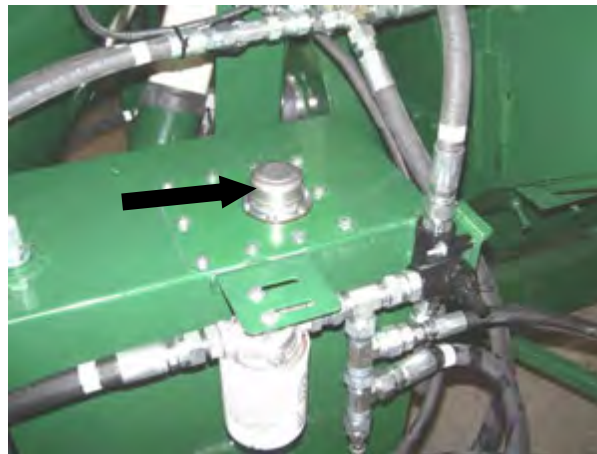
Figure 90 – Hydraulic Reservoir Cap (see Arrow)
