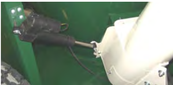
Figure 28 - Discharge Gate with Electric Actuator in closed position.
