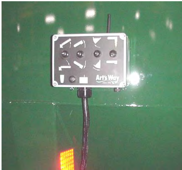
Figure 80 – Complete Control Box with internal Receiver as Backup Remote Control Box mounted on left rear side of mixer tank (for functions see Figure 90A).
