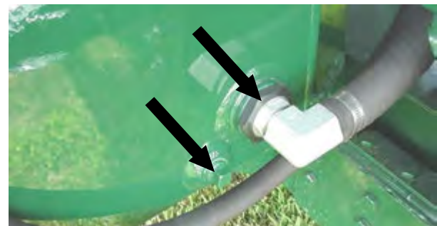
Figure 89 – Reservoir Strainer (on Right) and Drain (on Left)
