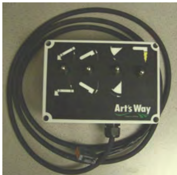
Figure 79 – Backup Remote Control Box (early units).
