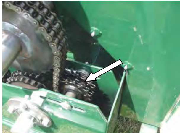
Figure 41 - Drive Chain Adjustment (Shield Removed for Clarity).
