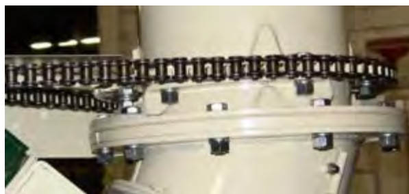
Figure 48 - Hydraulic Swing Adjustment (Shields Removed For Clarity).
