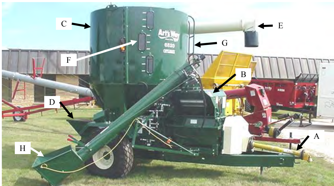
Figure 7 - Model 6520 CattleMaxx With Auger Feeder (A – PTO Driveline; B – Rollermill and Hopper; C – Mixing Tank; D – Supplemental Hopper; E – Discharge Auger; F – Viewing Windows; G – Ladder; H - Auger Feeder).
