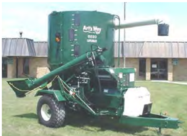
Figure 8 - Model 6520 CattleMaxx With Self-Contained Hydraulics, Auger Feeder.
