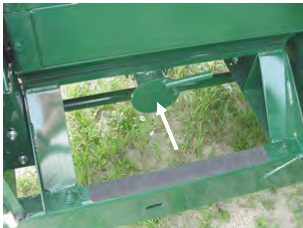
Figure 21 - Grain Inspection Trough.
