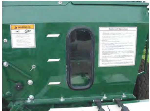
Figure 39 - Hopper Inspection Window.
