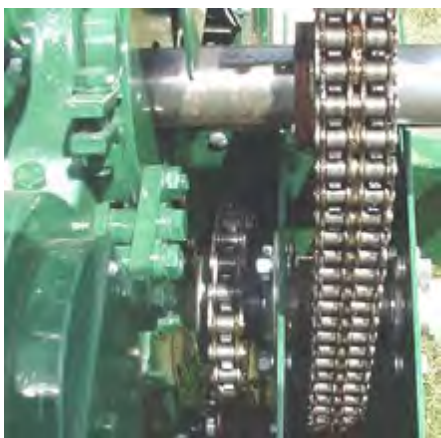
Figure 72 – Sprocket and Chain Alignment (shield opened for clarity).
