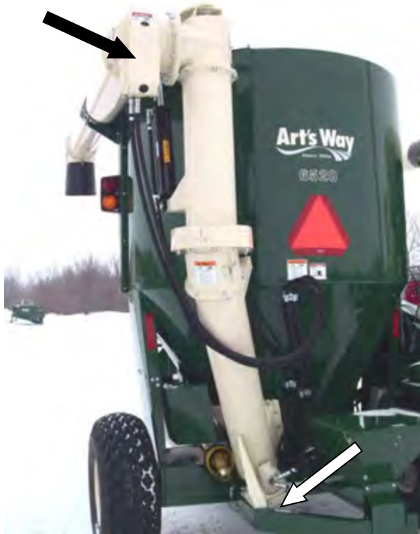
Figure 50 – Discharge Auger Drive Chain Locations (see arrows).
