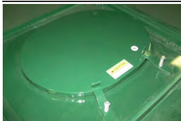
Figure 26 - Spring Loaded Tank Lid.
