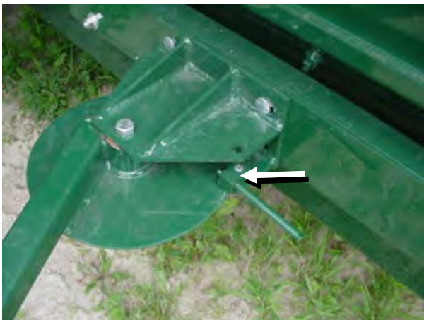
Figure 35 - Auger Feeder Swing Brake
