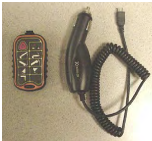
Figure 81A – Micro-Remote Control device with Charger (button functions same as Mini-Controller - Figure 88).
