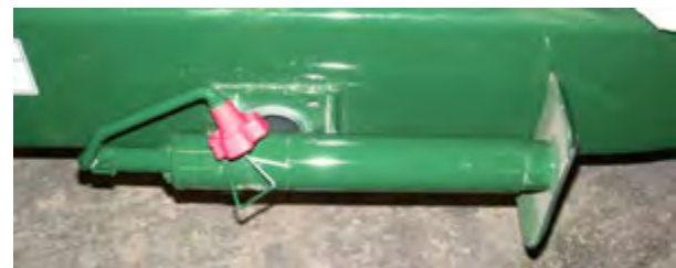
Figure 13 - Jack in Transport Position
