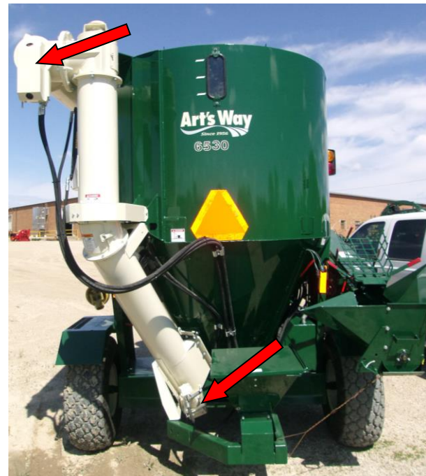
Figure 56 – Discharge Auger Drive Chain Locations (see arrows).
