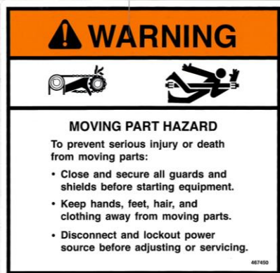
9. WARNING – Moving Part Hazard (467450)
