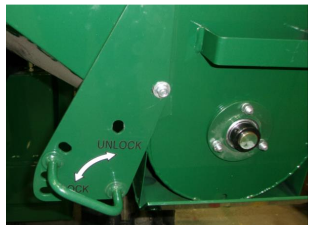
Figure 37 – Auger Feeder Latch Handle (shown in locked position).
