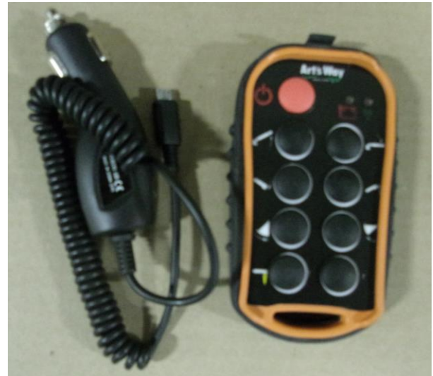
Figure 102 – Macro-Remote Control device with Charger.
