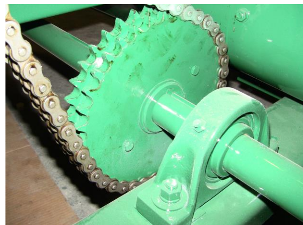
Figure 83 - Mixer Sprocket (Shields Removed For Clarity).
