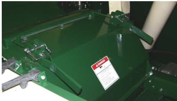
Figure 23 - Locking Pin and Latch on Hammer mill Door.
