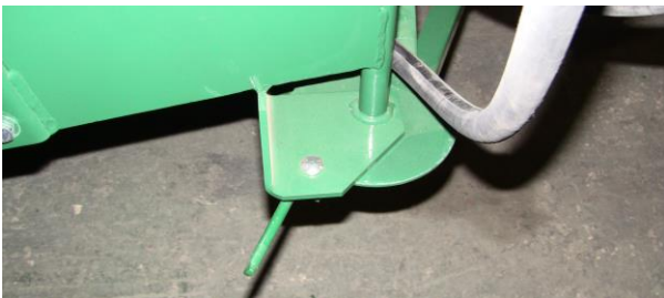
Figure 39 - Auger Feeder Swing Brake.
