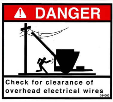
7. DANGER – Electrocutation Hazard (384000)
