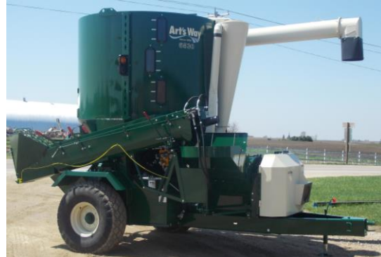
Figure 8 - Model 6530 With Self-Contained Hydraulics and Auger Feeder.
