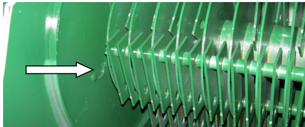
Figure 89 - Hammer Removal Inside Hammer mill, Hole to Remove Hammer mill Rods (Shields Removed For Clarity).
