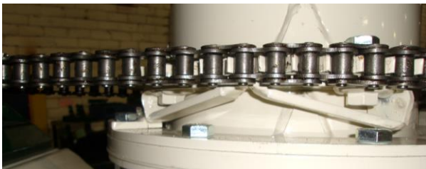
Figure 54 - Hydraulic Swing Adjustment (Shields Removed For Clarity).
