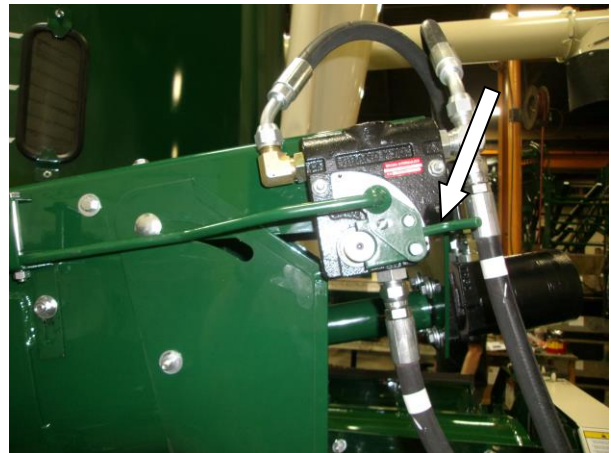
Figure 44 - Hydraulic Auger Feeder Control - shown in full on position (See Arrow).
