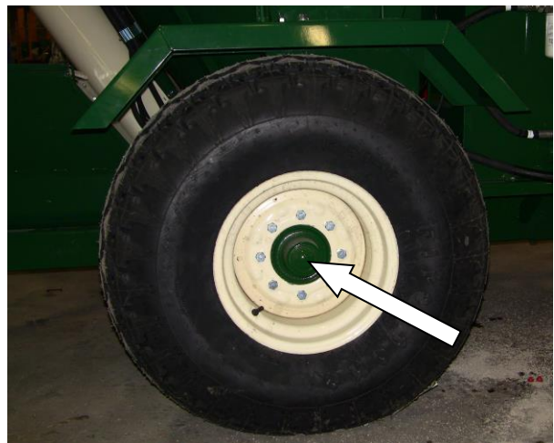
Figure 81 - Wheel Bearing Lubrication.
