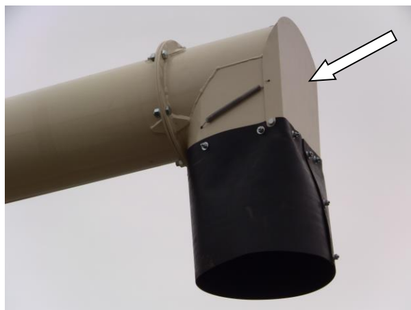
Figure 36 - Unloading Auger Hood.
