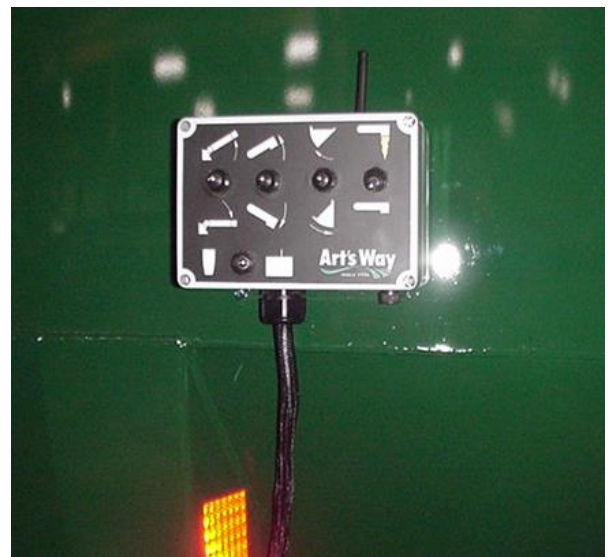
Figure 103 – Complete Control Box with internal Receiver mounted on left rear side of tank.
