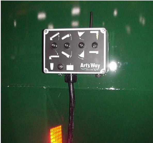
Figure 99 – Complete Control Box with internal Receiver as Backup Remote Control Box mounted on left rear side of mixer tank (for functions see Figure 104).
