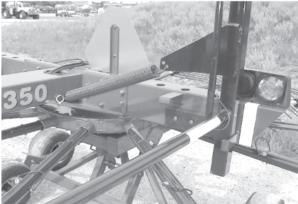
Guard in transport position (Delivery Side). Left Hand Delivery rake shown. Pull guard forward and down to unfold guard to field position. DO NOT operate rake in this position.
