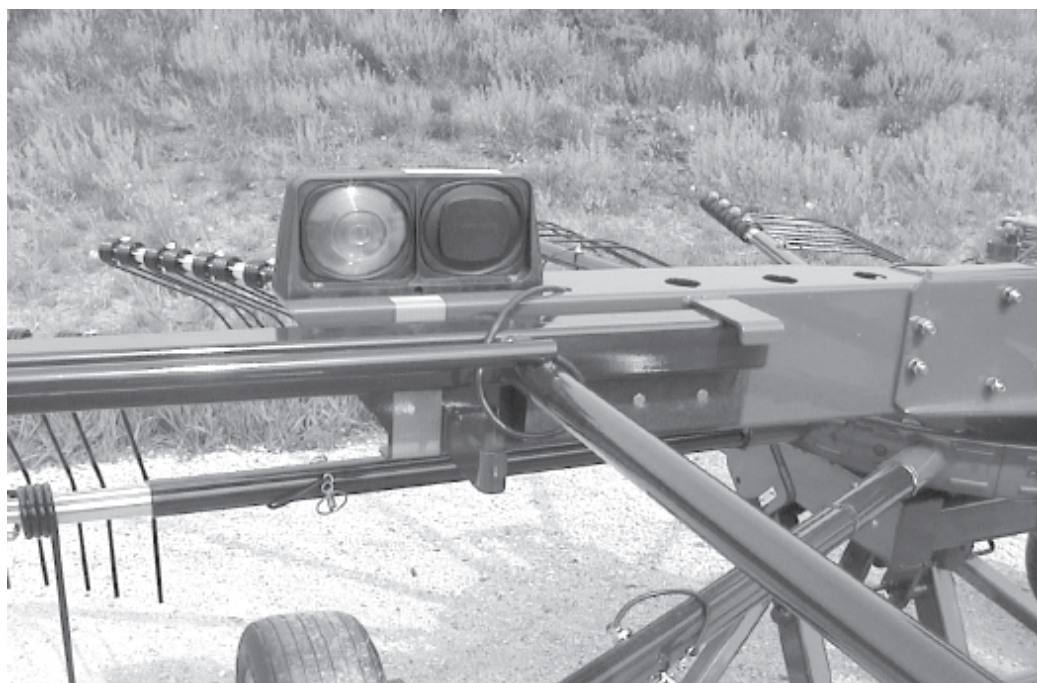
Guard in field position (Non Delivery Side). Left Hand Delivery rake shown. Pull guard forward and lift to fold guard to transport position.
