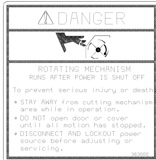
"DANGER" – ROTATING CUTTING MECHANISM THAT RUNS AFTER POWER IS SHUT OFF (P/N 363000)
