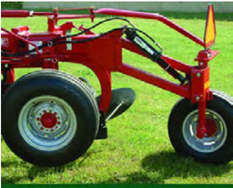
11L-15 load rating "F" PR steerable rear furrow wheel, 9.5L-15 8 PR gauge wheel
