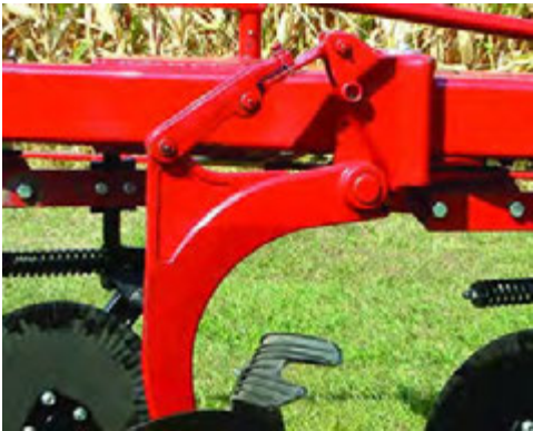
11L-15 load rating "F" PR steerable rear furrow wheel, 9.5L-15 8 PR gauge wheel
