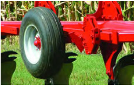
Rear gauge wheel automatically reverses its position as the bottoms rotate
