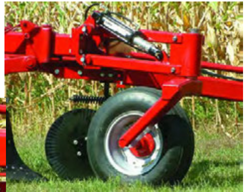
9.5L-15 12 PR tire castering front wheel
