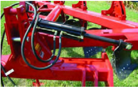
Heavy-duty frame and hydraulic rollover for dependable long life
