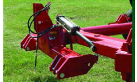
3-pt. cat II and III on 3-,4- and 5-furrow 3-pt. cat III and IV on 6 furrow
