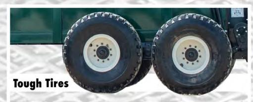
X Series Spreaders feature tandem axles with 16 R 20 tires. These allow you to pull the load smoothly behind your tractor without taking the field out with you. 600/50 R 22.5 flotation tires are available for decreased soil compaction in your fields and lower loading height.
