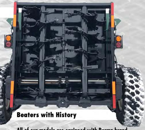
All of our models are equipped with Berma brand vertical beaters powered by dual 350 gear drive.s The X500 and X700 uses SRT8 while the X900 uses SRT18 sized beaters. These beaters combined with our unique spacing and positioning provide the best spread pattern in the industry.
