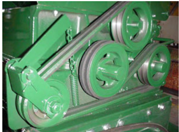
Figure 8 - Belt Adjustment (Shields Removed For Clarity).
