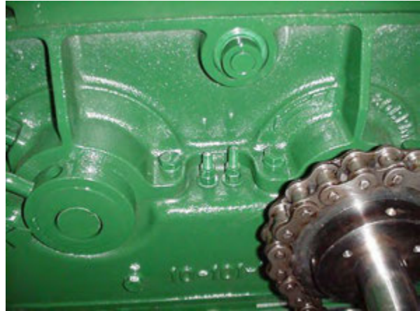
Figure 7 - Roll Scraper Adjustment Bolts
