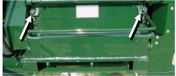
Figure 11 - Grain Control Gate Lubrication (2 Zerks And Slide Guides).
