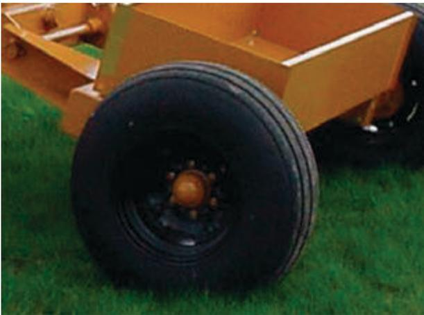
Figure 14. Hub and Wheel Bearing.
