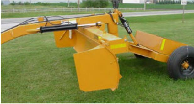
Figure 7. Box ends locked in down position.
