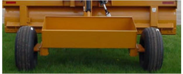
Figure 9. Sandbox on rear frame assembly.
