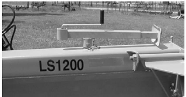
Figure 11. Jack storage on moldboard.
