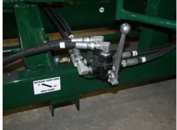
Figure 41 - Hydraulic Auger Feeder Selector Valve Lever Is In The Out Position - Auger Feeder.
