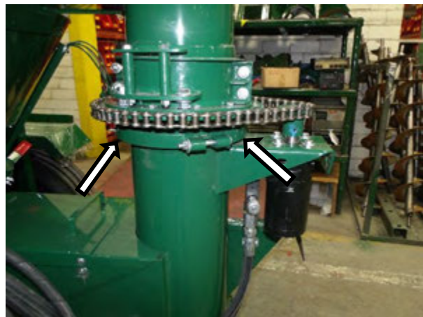
Figure 81 - Swivel Clamp Area, Discharge Auger (Shield Removed For Clarity).
