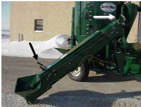
Figure 39 - Hydraulic auger feeder controls. (See arrows)
