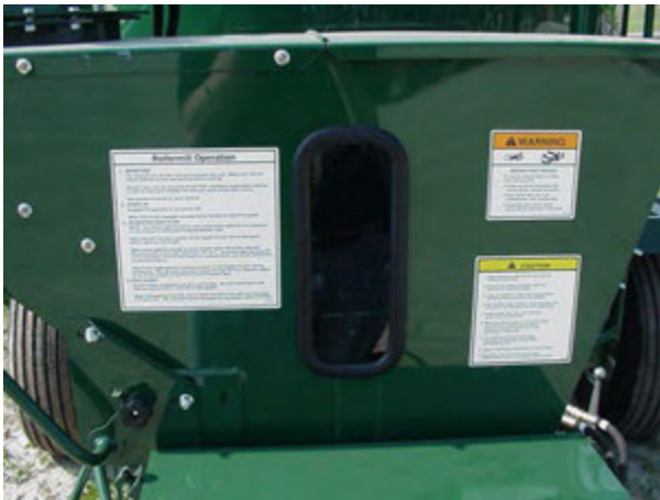
Figure 143 - Hopper Inspection Window.
