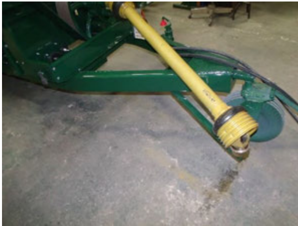
Figure 66 - PTO Driveline (Shield Removed For Clarity).
