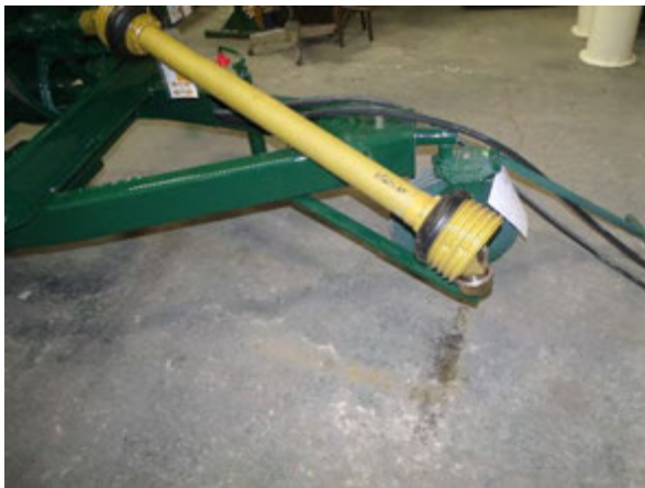
Figure 162 - PTO Driveline (Shield Removed For Clarity).
