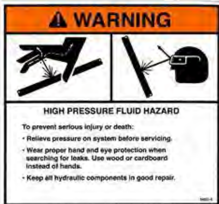
8. WARNING –High Pressure Fluid Hazard (346310)
