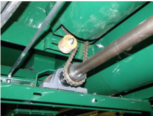
Figure 43 - Discharger Auger Drive Chain (Shields Removed for Clarity).
