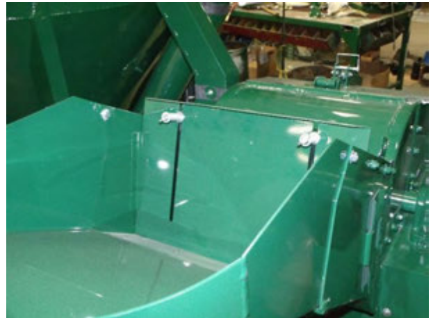
Figure 17 - Feed Gate At Throat Of The Hammermill.
