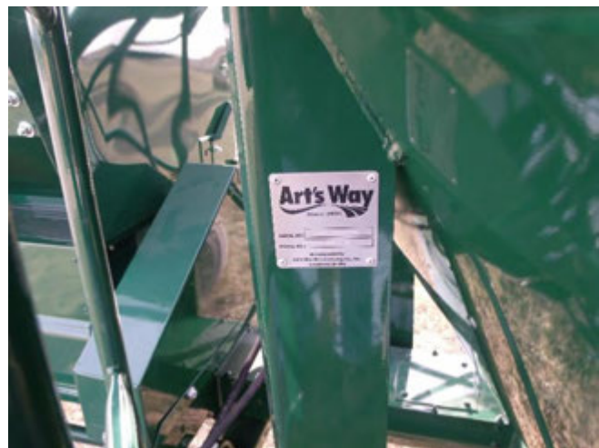
Figure 1 - Serial Number Placard Location. Left front tank support.
