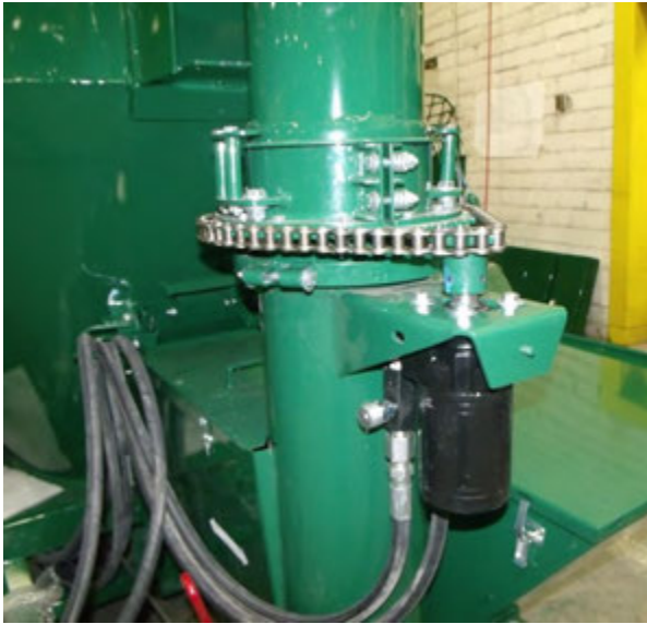
Figure 153 - Hydraulic Swing Adjustment (Shields Removed For Clarity).
