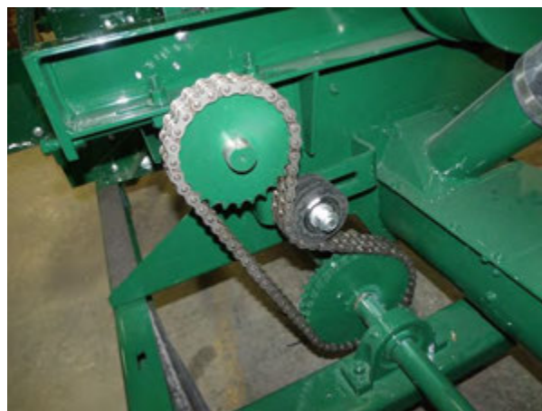
Figure 90 – Jack Shaft to Mixing Auger Sprockets (Shields Removed For Clarity).
