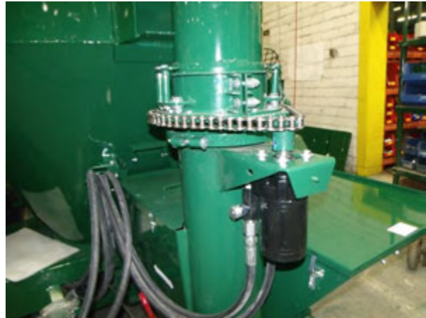
Figure 60 - Hydraulic Swing Adjustment (Shields Removed For Clarity).
