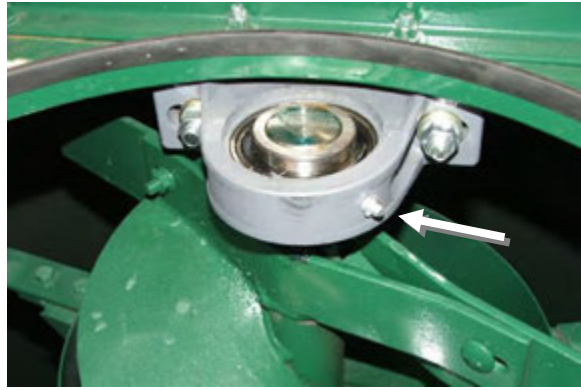
Figure 79 - Upper Vertical Mixing Auger Bearing.
