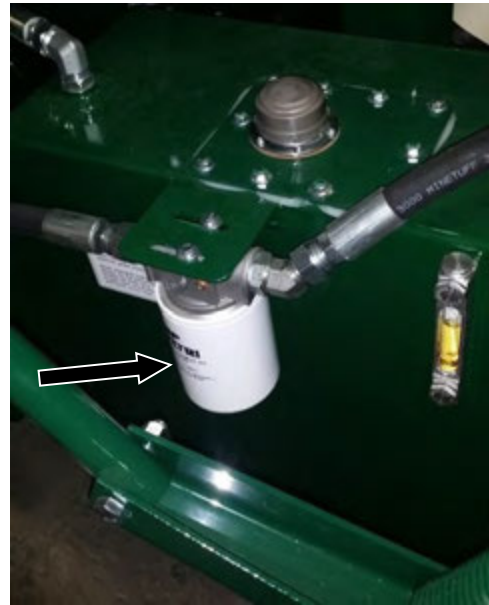
Figure 88 – Reservoir Filter (See Arrow).
