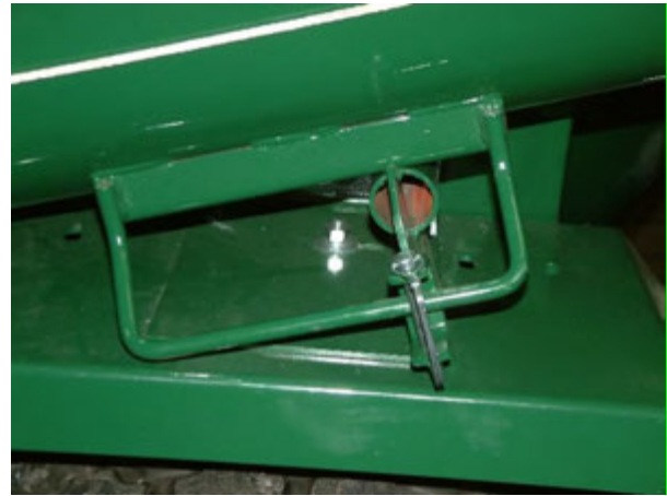
Figure 33 - Auger Feeder Latch Handle (Shown in Locked Position).
