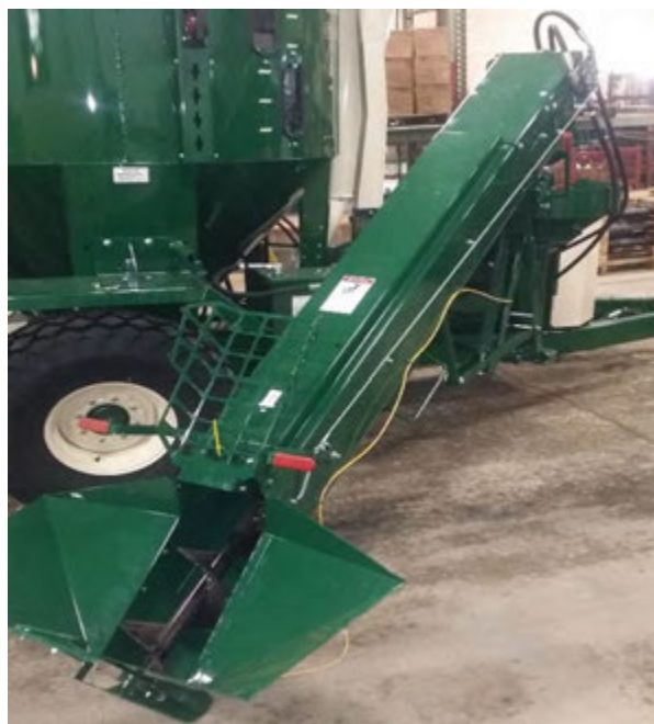
Figure 34 - Auger Feeder Operation (Grate in Lifted Position).
