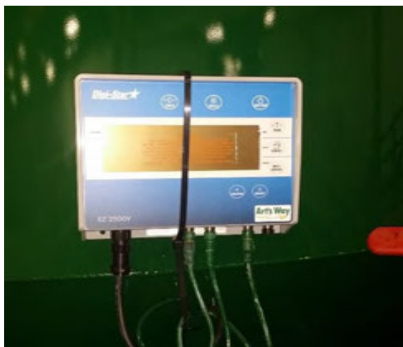
Figure 91 - Scale Head Attachment (EZ2500V Shown).
