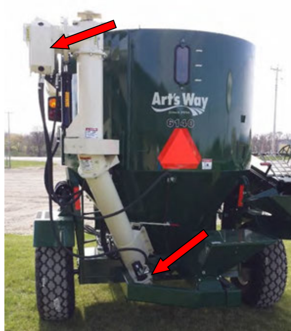
Figure 51 - Discharge Auger Drive Chain (See Arrows).
