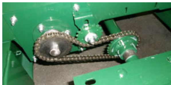
Figure 76 – Mill To Mixer Sprocket (Shields Removed For Clarity).
