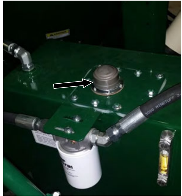
Figure 90 – Hydraulic Reservoir Cap (See Arrow)
