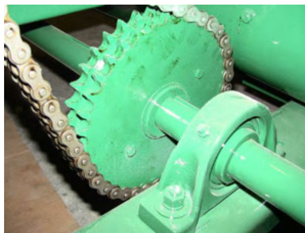
Figure 75 - Mixer Sprocket (Shields Removed For Clarity).
