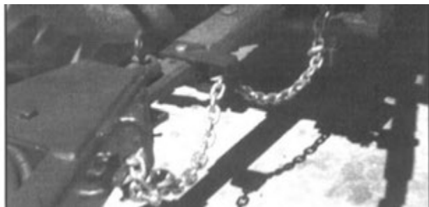
Figure 14 - Grinder Attached To The Tractor With Safety Chain.
