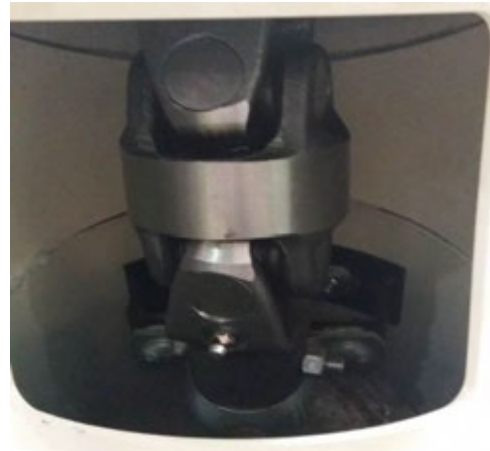
Figure 71 – Discharge U-Joint (Door Removed for Clarity).
