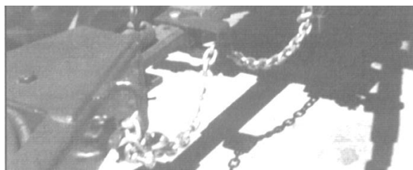
Figure 14 - Attached to the Tractor with Safety Chain.
