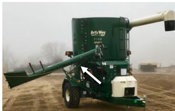
Figure 39 – Auger Feeder Counter Balance Spring
