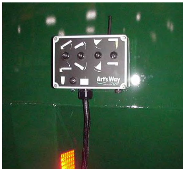
Figure 85 – Complete Control Box with Internal Receiver.
