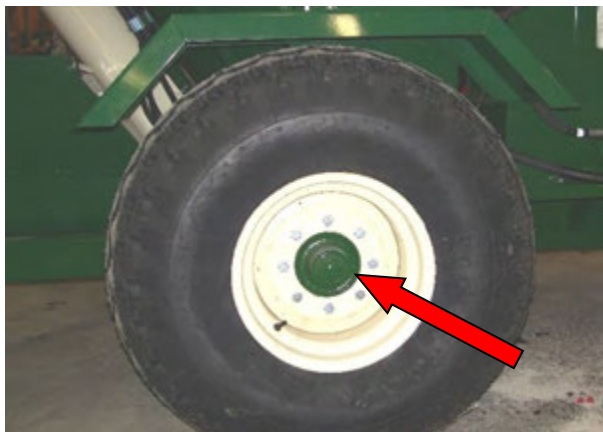
Figure 76 - Wheel Bearing Lubrication.
