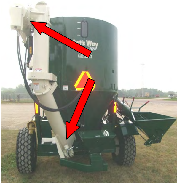
Figure 52 – Discharge Auger Drive Chain Locations (see arrows).
