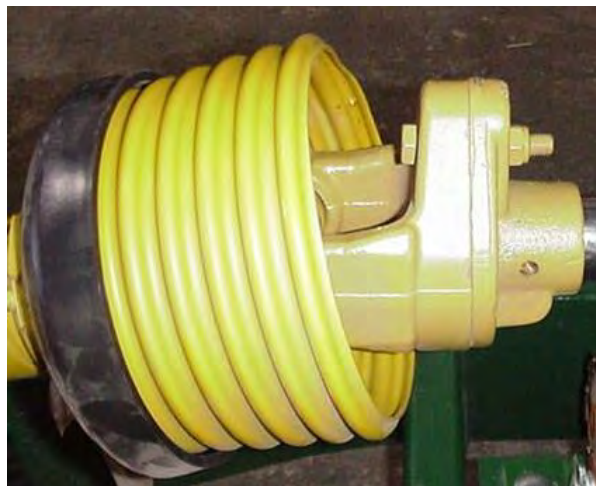
Figure 18 - PTO Driveline Shear Clutch
