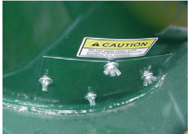
Figure 23 - Tank Cone Clean-Out Door (Left-Hand Side Shown).
