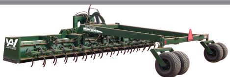
Land Planes are the only way to insure even distribution of rainfall or irrigation. Water pockets can be eliminated by utilizing the natural slope of the field. On rolling ground, land smoothing improves surface drainage thereby controlling erosion.
