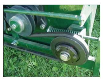
Figure 16. – Harvester Grab Roller Forward Belt Drive Spring Tensioner
