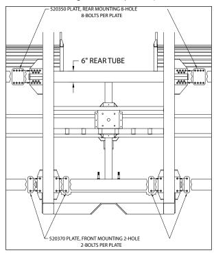
Figure 92. - Mounting Plate Details
