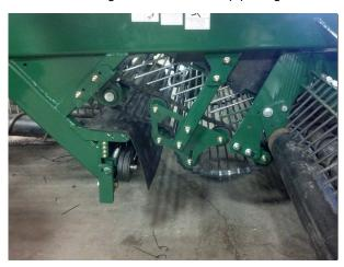
Figure 93. - Short Conveyor Attachment Point
