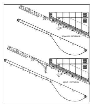
Figure 98. - Draper Chain Routing
