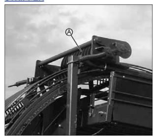
Figure 73. - Wheel Elevator Stripper
