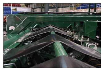
Figure 59. - Header Protective Rubber Covers
