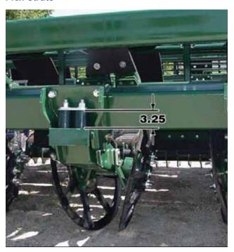
Figure 55. - Header Lifter Wheel Flex Struts
