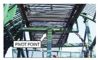
Figure 44. - Transfer Conveyor Pivot System
