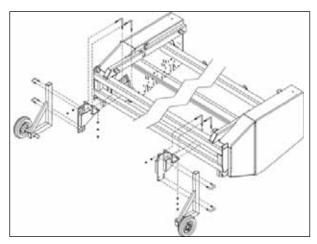
Figure 95. - Wheel Mounts, Front (Optional)
