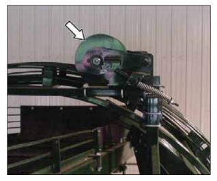
Figure 101. - Wheel Elevator Stripper
