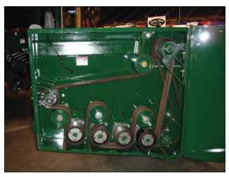
Figure 13. – Harvester Right-Hand Belt Drive (Rear Grabroll Option Shown)
