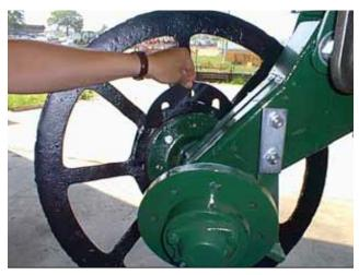
Figure 52. - Header Lifter Wheel Width Shims
