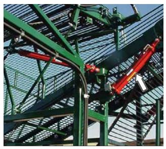
Figure 48. – Truck Boom Conveyor Hydraulic Cylinders
