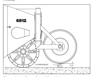
Figure 64. - Front Gage Wheel Height
