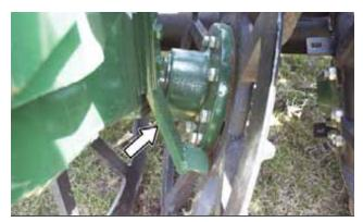
Figure 28. - Lifter Wheel Scrapers
