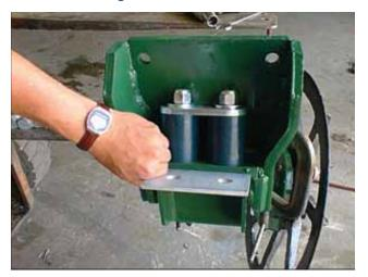
Figure 53. - Header Lifter Wheel Height Shims
