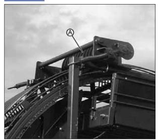
Figure 73. - Wheel Elevator Stripper
