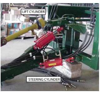
Figure 24. - Harvester Lift & Steering Cylinders
