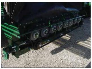
Figure 38. - Harvester Grab Rollers Front Drive
