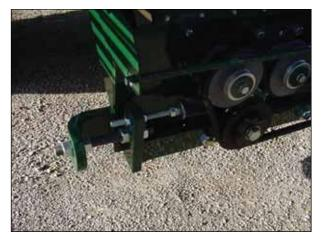
Figure 67. – Harvester Grabrollers - Single Point Adjustment (Front)
