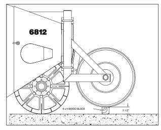
Figure 96. - Front Header Wheels Height
