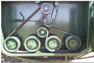
Figure 37. - Harvester Rear Belt Drive System
