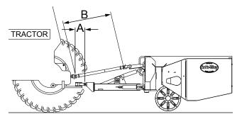
Figure 22. - Drawbar And PTO Specifications
