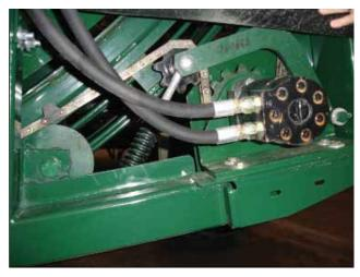
Figure 19. – Wheel Elevator Motor Sprocket and Drive Chain
