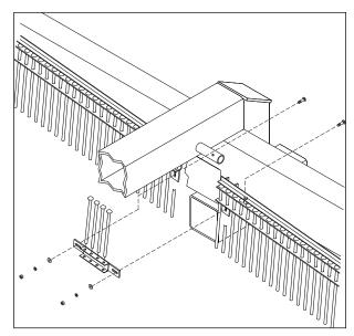
Figure 85. - Axle Grate Installation
