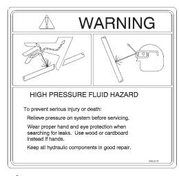
8 P/N: 366310 Decal, Warning, High Pressure Fluid Hazard
