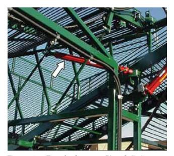
Figure 45. - Transfer Conveyor Pivot Cylinder
