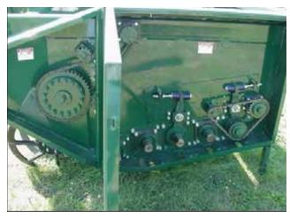
Figure 32. – Header Left-Hand Drive. (8 Row 22 Header Shown)
