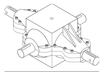
Figure 11. - Harvester Gearbox
