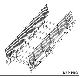
Figure 18. – Truck Conveyor Sprocket and Drive Chain
