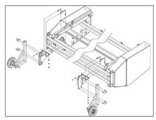
Figure 95. - Wheel Mounts, Front (Optional)
