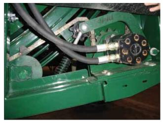
Figure 19. – Wheel Elevator Motor Sprocket and Drive Chain
