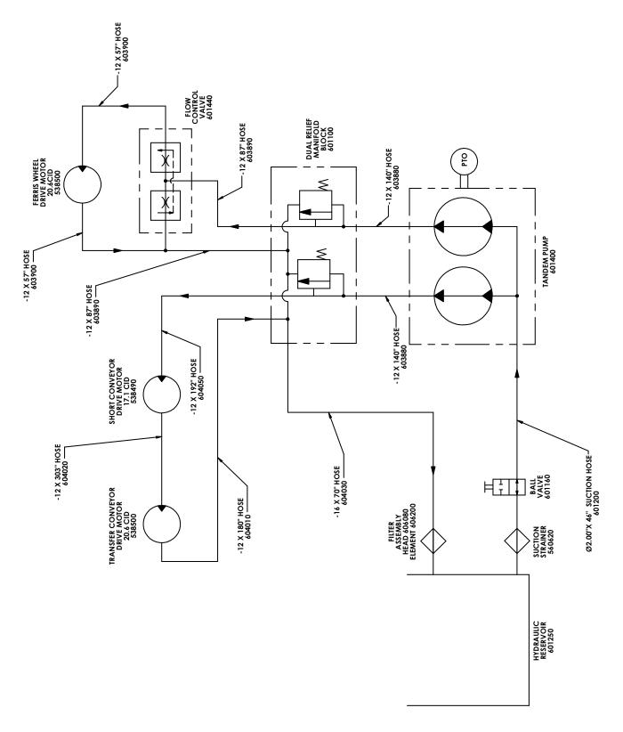
Figure 77. - Harvester Self-Contained Hydraulic System
