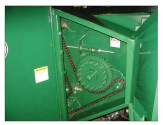
Figure 12. – Header Left-Hand Paddle Shaft Chain/ Drive
