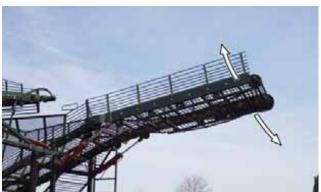
Figure 46. – Truck Boom Conveyor With Boom Extended
