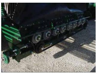
Figure 38. - Harvester Grab Rollers Front Drive
