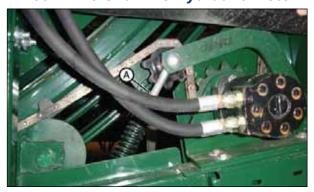
Figure 70. – Wheel Elevator Sprocket, Chain Drive, and Roller
