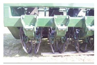
Figure 27. - Header Lifter Wheels
