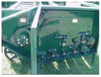
Figure 14. – Harvester Left-Hand Chain and Gear Drive. (6 Row 30 And 8 Row 22)
