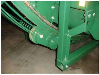
Figure 41. – Wheel Elevator Roller (Left-Hand Side)
