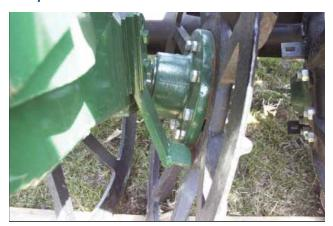
Figure 54. – Header Lifter Wheel Scraper Adjustments
