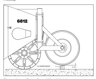
Figure 64. - Front Gage Wheel Height
