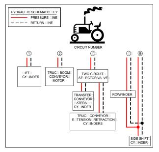
Figure 102. - Tractor/Harvester Hydraulic System
