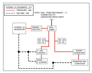
Figure 103. – Harvester Self-Contained Hydraulic System
