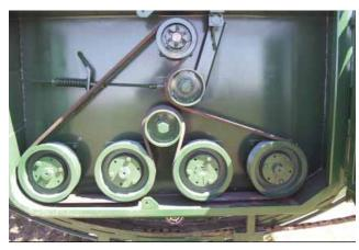
Figure 15. – Harvester Rear Belt Drive System and Pump Drive
