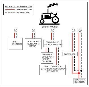
Figure 102. - Tractor/Harvester Hydraulic System
