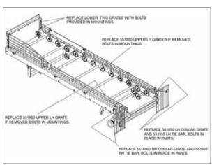
Figure 100. - Grates For Transfer Elevator
