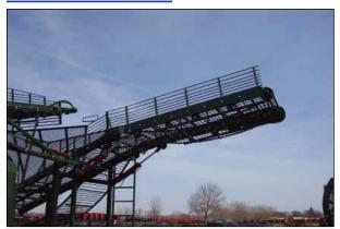
Figure 74. - Truck Boom Conveyor
