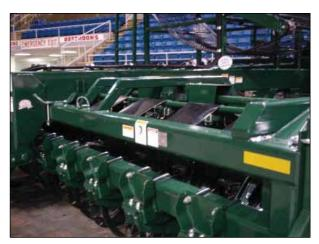
Figure 87. - Header Drive Shafts
