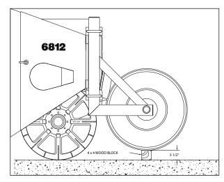
Figure 96. - Front Header Wheels Height
