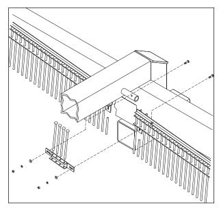
Figure 85. - Axle Grate Installation
