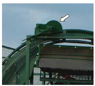
Figure 42. - Wheel Elevator Stripper
