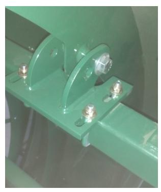
Figure 71. - U-Bolts & Pivot Bracket
