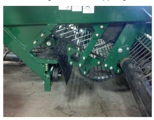
Figure 93. – Short Conveyor Attachment Point
