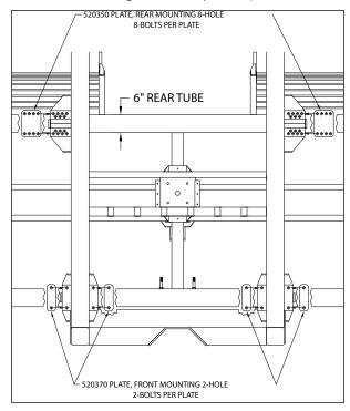
Figure 92. - Mounting Plate Details
