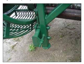
Figure 68. – Harvester Grabrollers - Single Point Adjustment (Back)
