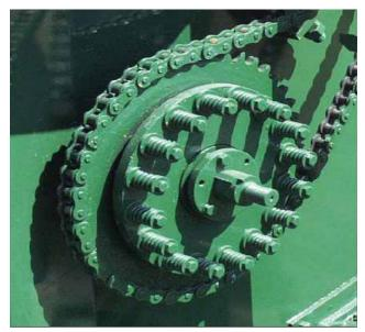
Figure 61. - Friction Slip Clutch
