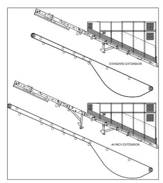
Figure 98. - Draper Chain Routing
