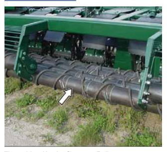
Figure 31. - Header Conveyor Rollers
