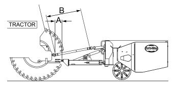
Figure 22. - Drawbar And PTO Specifications
