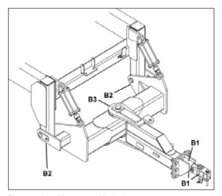
Figure 79. - Harvester Hitch Area
