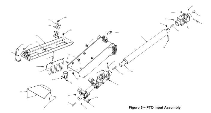
Install the support assembly to the frame and secure using 5/8 X 2 HFH, flange-nyloc-nuts (9,12). Adjust the short lower shaft in bearings with no binding and lock collars on bearings.
