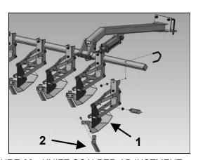
FIGURE 22 - KNIFE SCALPER ADJUSTMENT
