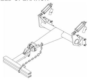
Figure 11 - Safety Chain Attachment.
