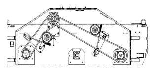
Figure 15 - Open Shield, LH Drive.
