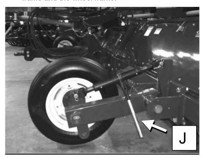
Figure 8 - Wheel and Tire Assembly Installation
