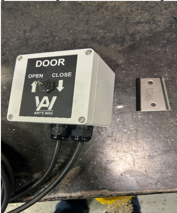
Figure 29 – Tractor Hydraulics Actuator Control Box and Mounting Parts.
