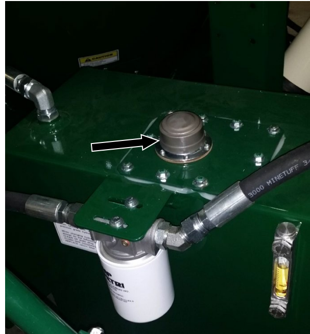
Figure 90 – Hydraulic Reservoir Cap (See Arrow)
