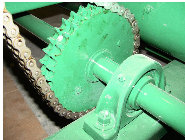
Figure 75 - Mixer Sprocket (Shields Removed For Clarity).
