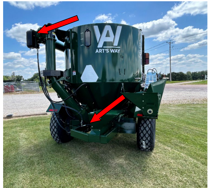
Figure 51 - Discharge Auger Drive Chain (See Arrows).
