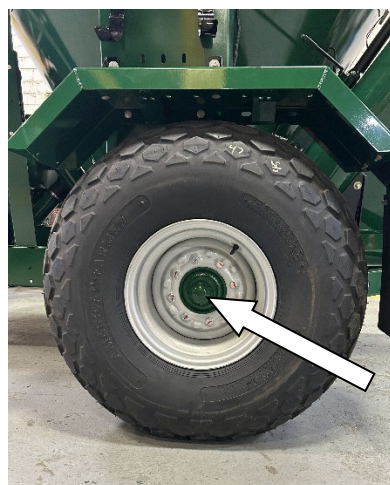
Figure 73 - Wheel Bearing Lubrication.
