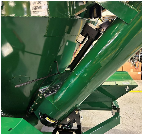
Figure 28 - Discharge Gate with Electric Actuator in closed position.
