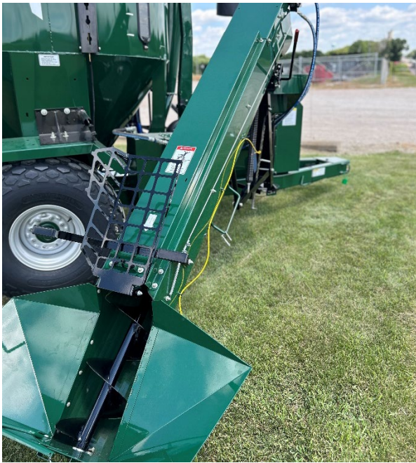
Figure 34 - Auger Feeder Operation (Grate in Lifted Position).
