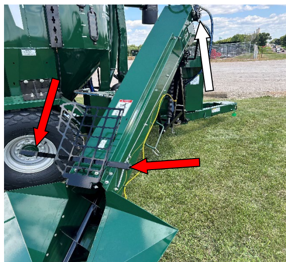
Figure 39 - Hydraulic Auger Feeder Controls (Shown in Off and Transport Position): Throttle Controls (White Arrow) and Emergency Shutoff (Red Arrows).
