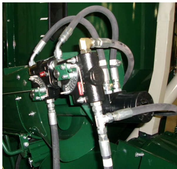
Figure 95 - Roll Feed and Auger Feeder Flow Control Valves.
