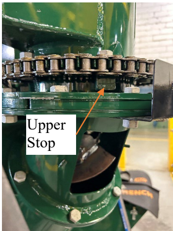
Figure 50 - Rear Swivel Stop (Shields Removed for Clarity).
