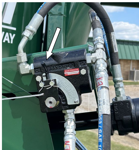
Figure 40 - Hydraulic Auger Feeder Control (Shown in Full Off Position) (See Arrow).
