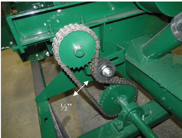
Figure 42 - Drive Chain Adjustment (Shields Removed for Clarity).
