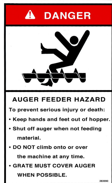
6. DANGER – Auger Feeder Hazard (383990)
