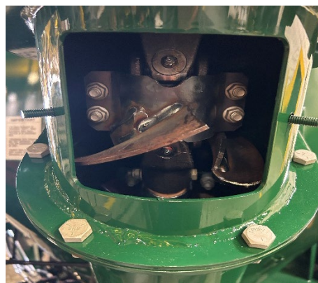
Figure 71 – Discharge U-Joint (Door Removed for Clarity).
