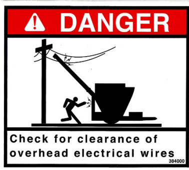
7. DANGER – Electrocutation Hazard (384000)
