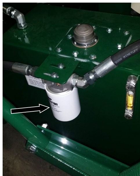
Figure 88 – Reservoir Filter (See Arrow).
