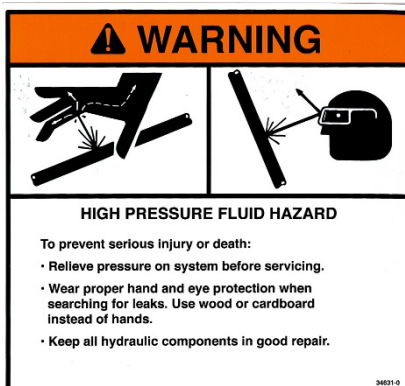
11. WARNING –High Pressure Fluid Hazard (346310)
