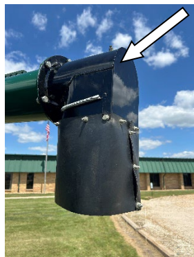
Figure 32 - Unloading Auger Hood.
