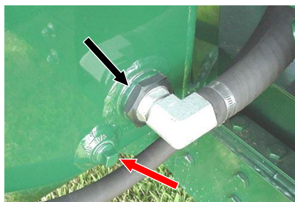
Figure 89 – Reservoir Strainer (Black Arrow) and Drain Plug at Front of Reservoir Tank (Red Arrow).
