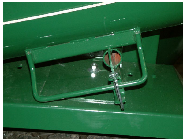
Figure 33 - Auger Feeder Latch Handle (Shown in Locked Position).
