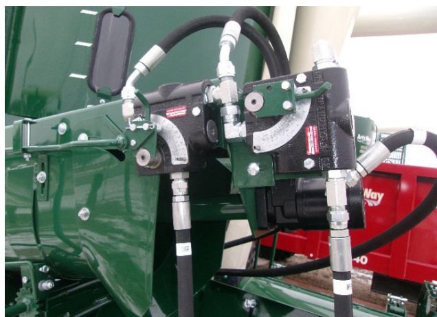
Figure 103 - Roll Feed and Auger Feeder Flow Control Valves.
