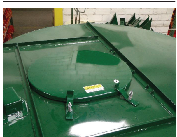
Figure 126 - Spring Loaded Tank Lid.
