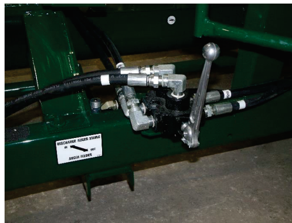
Figure 41 - Hydraulic Auger Feeder Selector Valve Lever Is In The Out Position - Auger Feeder.
