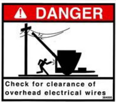
5. DANGER - Electrocutation Hazard (384000)
