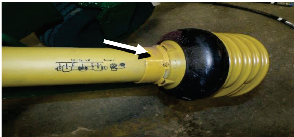
Figure 163 - Plastic Shaft Bearings (See Arrow).
