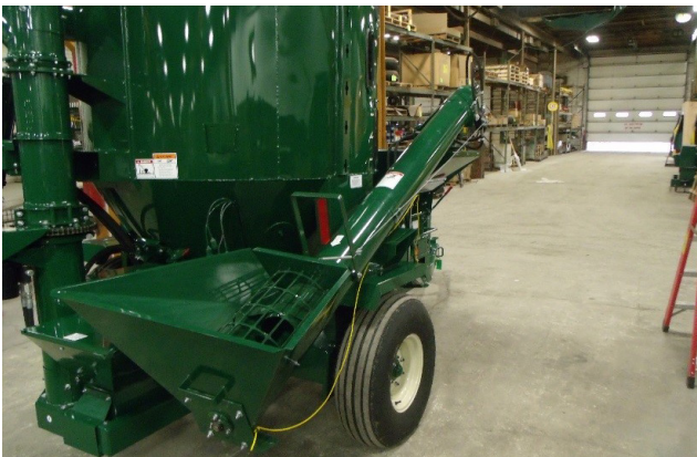
Figure 140 - Auger Feeder Positioner And Spring Adjustment (A - Spring; B - Positioner Handle; C - Positioner Lock).
