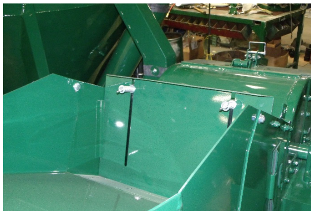
Figure 17 - Feed Gate At Throat Of The Hammermill.
