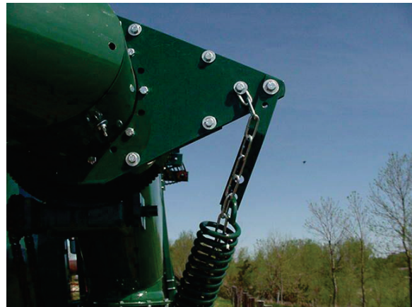
Figure 54 - Lift Assist Spring Adjustment Bolts
