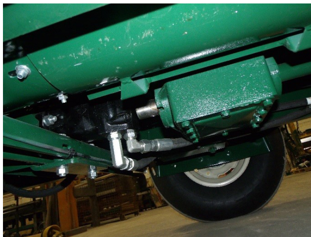
Figure 57 - Lower Discharge Motor (First Section)
