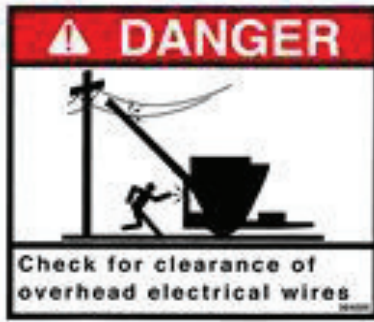
7. DANGER – Electrocutation Hazard (384000)
