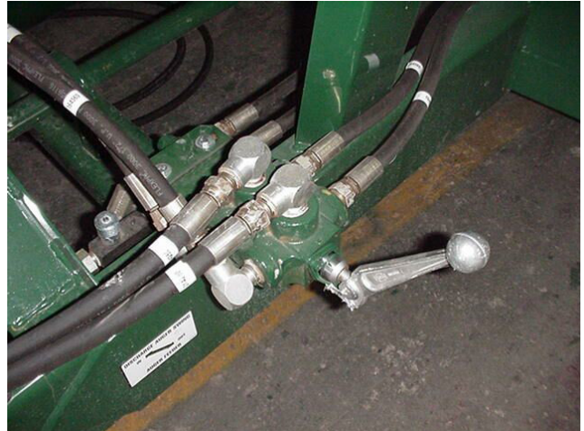
Figure 142 - Hydraulic Auger Feeder Selector Valve Lever Is In The Out Position - Auger Feeder).
