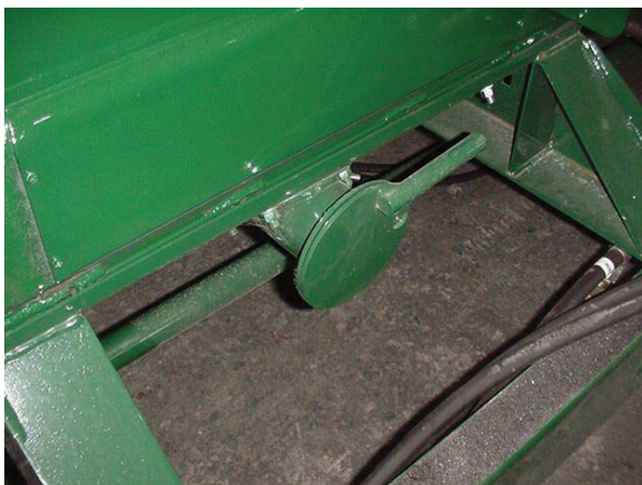
Figure 121 - Grain Inspection Trough.
