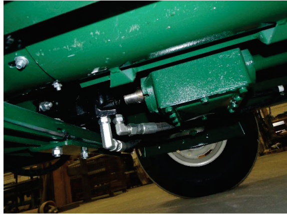
Figure 158 - Lower Discharge Motor (First Section)
