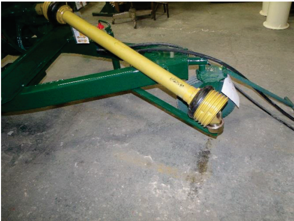
Figure 162 - PTO Driveline (Shield Removed For Clarity).
