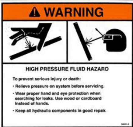
8. WARNING –High Pressure Fluid Hazard (346310)
