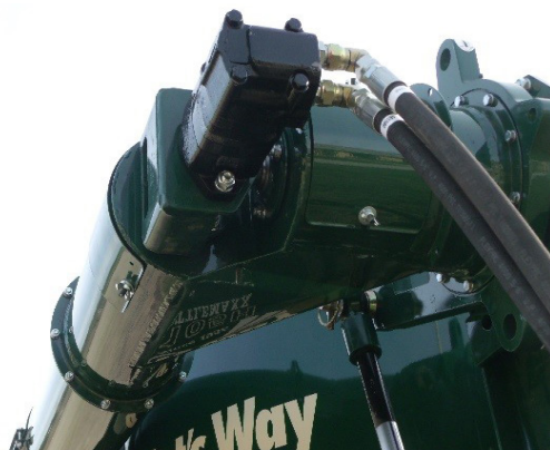
Figure 55 - Upper Discharge Motor (Unload)
