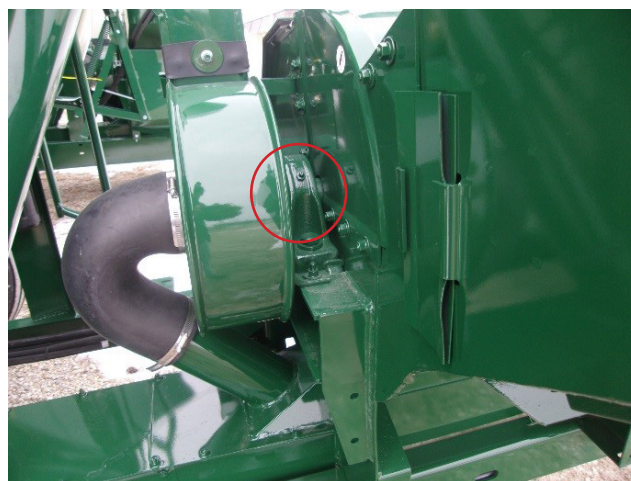
Figure 69 - Cylinder Shaft Bearing (See Circle) (Shields Removed For Clarity).
