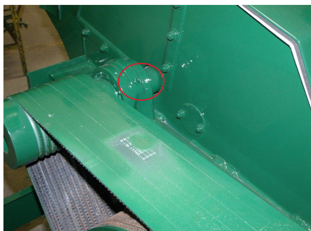
Figure 68 - Cylinder Shaft Bearing (See Circle) (Shields Removed For Clarity).
