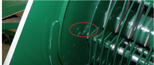
Figure 94 - Hammer Removal Inside Hammermill, Hole To Remove Hammermill Rods (Shields Removed For Clarity).
