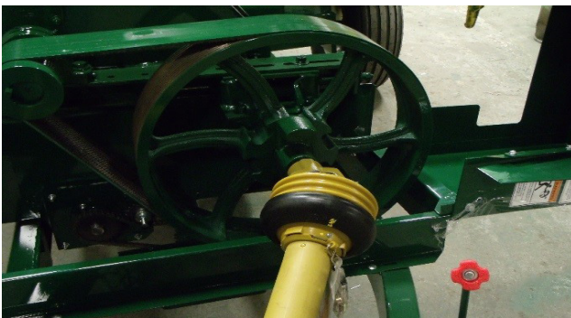
Figure 14 - Large Pulley - 540 RPM (Shields Removed For Clarity [-Ø22-5/8"]).
