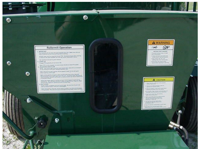
Figure 143 - Hopper Inspection Window.
