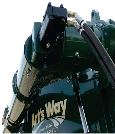
Figure 156 - Upper Discharge Motor (Unload)
