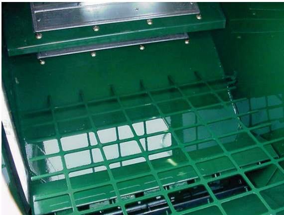
Figure 148 - Removing Magnet To Check Roll Spacing.
